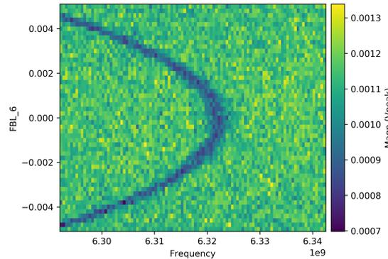
Figure 3.8: This is a Qubit DAC scan. It is a series of spectroscopy measurements in a specified range, repeated while varying the current on a flux line. This causes the qubit frequency to vary. The goal of this measurement is to extract the sweet spot, where the qubit is first order insensitive to flux noise. This is at the vertical part of the curve. The qubit frequency is expected to be a cosine function of the applied flux. Around the sweet spot, it can be approximated with a parabola.
