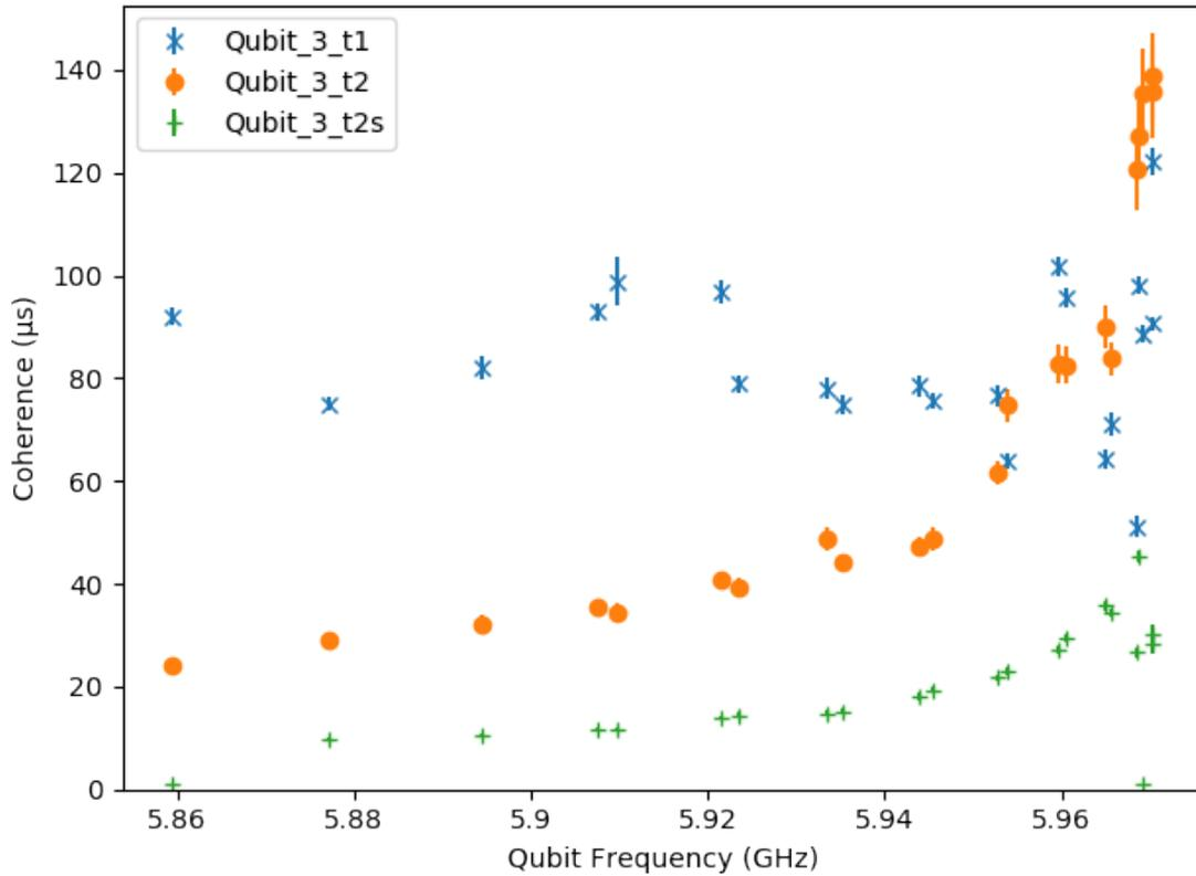
Figure 3.17: This is an example of a set of coherence measurements with varying frequencies on qubit 3. Every point represents a single measurement. This already clearly shows the quick reduction in  $T_2$  when moving away from the sweet spot.  $T_1$  does not vary more than it would in a time trace where the frequency is not varied.
