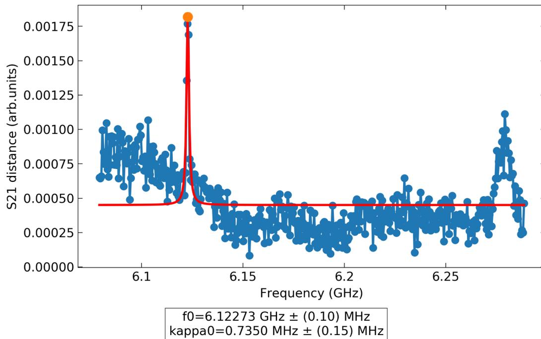
Figure 3.15: A high-power spectroscopy scan where both the 01 and 02 transitions are visible. From the width of the 01 transition it is clear that the power is a lot higher than in a regular spectroscopy measurement. The 02 peak is still quite narrow, and so the frequency found by the peak finder can be used to quite accurately predict the anharmonicity of the qubit.
