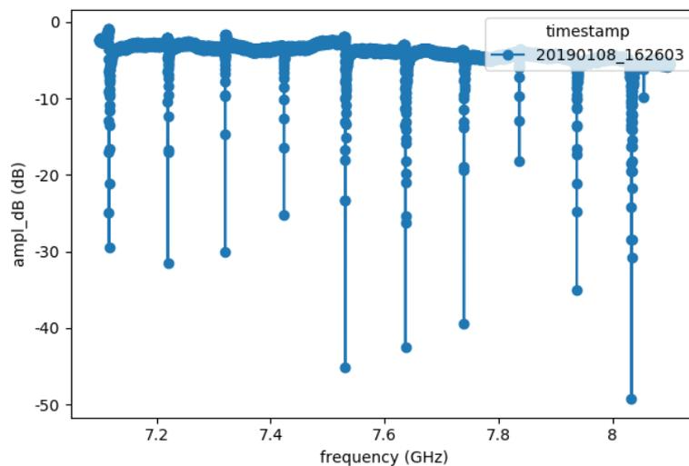
Figure 3.1: An overview scan of all the resonators. All ten qubit resonators are evenly spaced and clearly visible. The small peak on the right is the test resonator, which has a far weaker coupling to the feed line, resulting in a more shallow dip.
