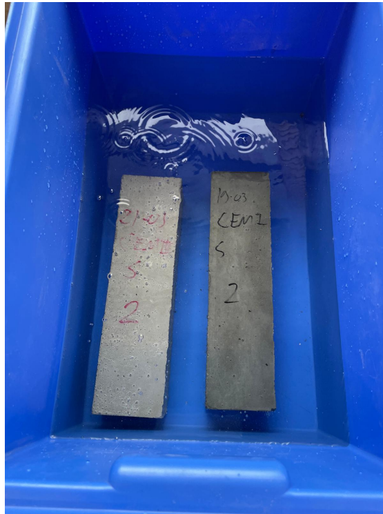
Figure 6.15: Absorption test setup
