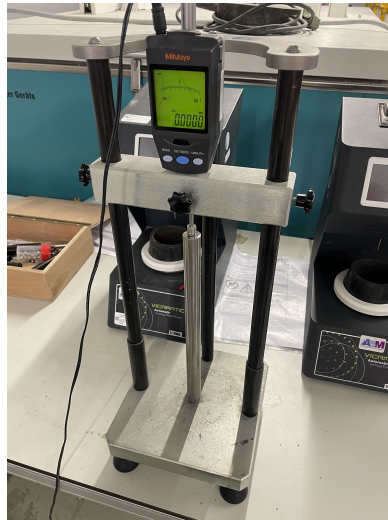
Figure 6.3: Shrinkage test setup
