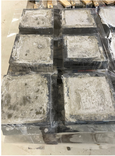
Figure 6.5: Concrete cubes for compression test
