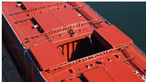
Figure 3.8: Side-rolling hatch cover [34].
