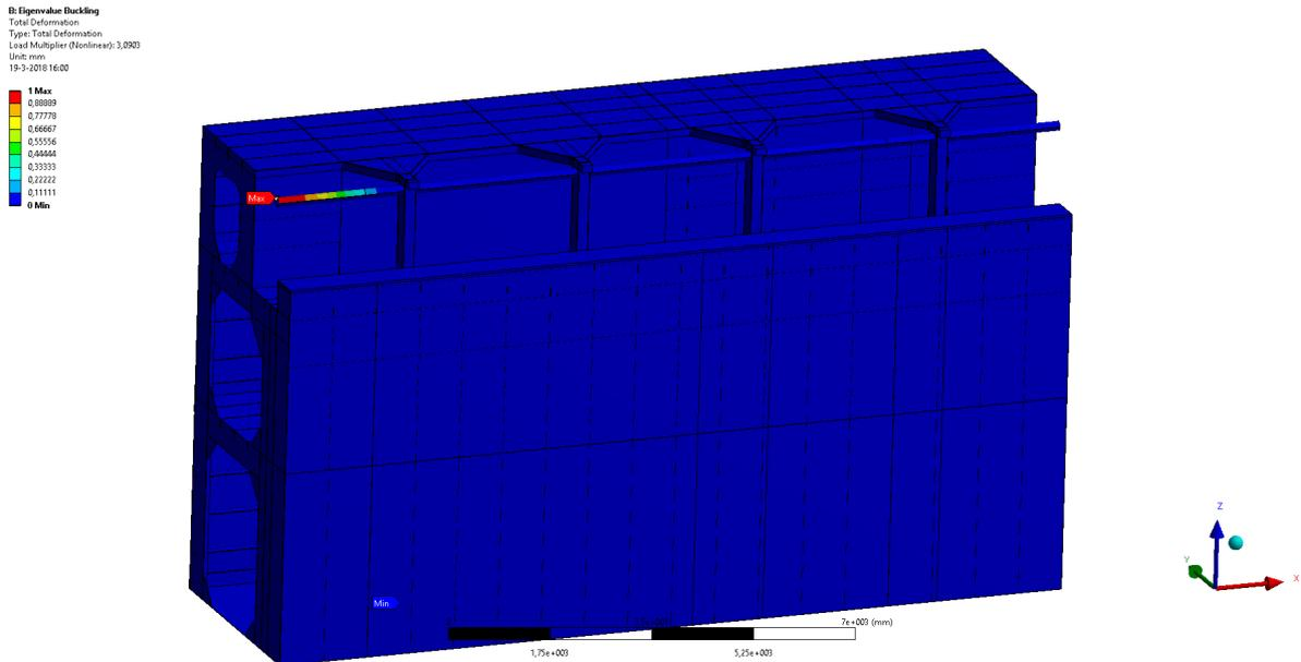
Figure F.18: Buckling analysis seafastening system starboard.
