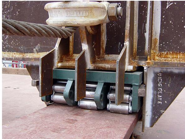
Figure 3.4: Hilman rollers propelled by a strand [57].
