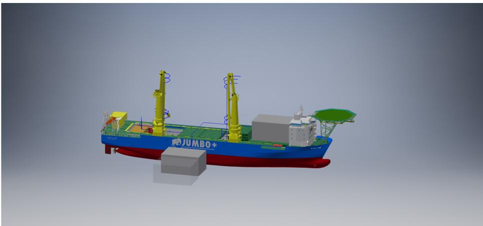
(d) Cargo shifted to position 1&2, hatch 7& 8 are brought to position 4&5. Hatches 3,4,5,6 are stored at location 3.
