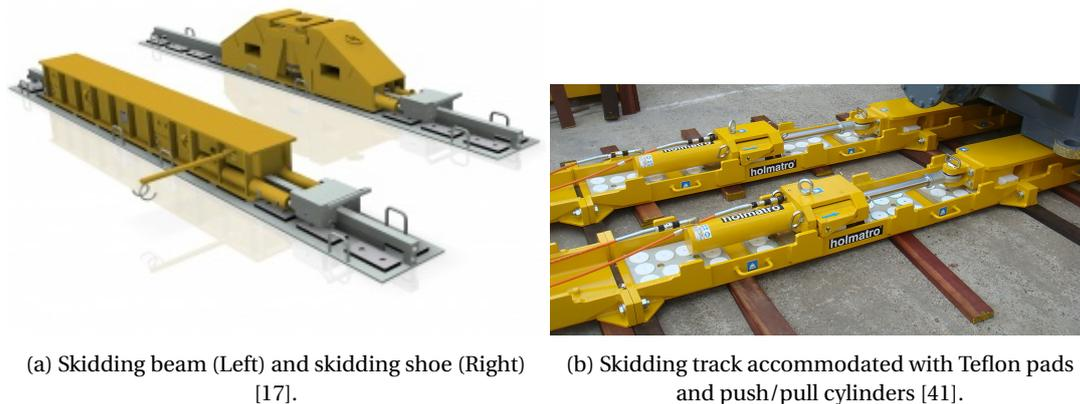
Figure 3.3: Teflon based skidding operation.
