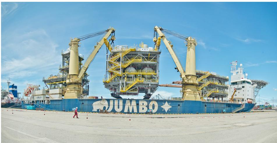
Figure 1.7: Cargo loaded on hatch covers on a J1800-class vessel.
