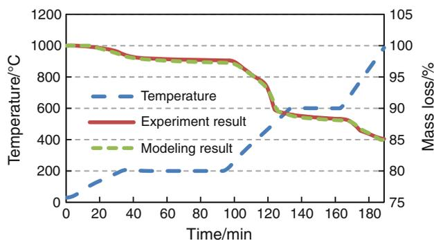
**Fig. 7** Comparison of mass loss measured by thermogravimetry and mass loss curve predicted by kinetics model under complex temperature program
