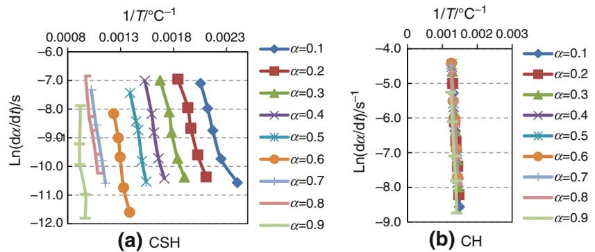
**Fig. 5** Activation energy and  $\ln A$  determined by isoconversional method
