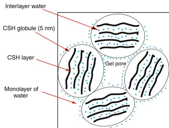
**Fig. 6** A schematic of globulous structure of CSH gel
