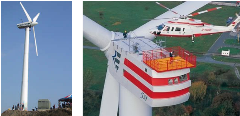
Figure 1.1: Different HAWT machines - ( left ) Stall-controlled Vestas V17 - ( right ) Pitch-controlled Enercon E126
