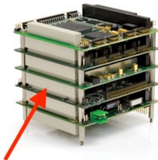
(b) Picture of the PC/104 connector (gray) in a satellite stack.
