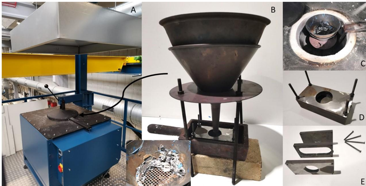
Figure 3. Melting Oven. A: The induction furnace for melting of the Zamak laryngoscope blades. B: All-in-one casting setup, a bowl with grate placed in the melting oven. C: Top bowl with filter allows only the Zamak to pass. D: Cast with riser. E: Exploded view cast with riser.
