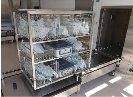
Picture 2: Steriliser batch with FFP2 masks for decontamination together with other loads suitable for this sterilisation process
