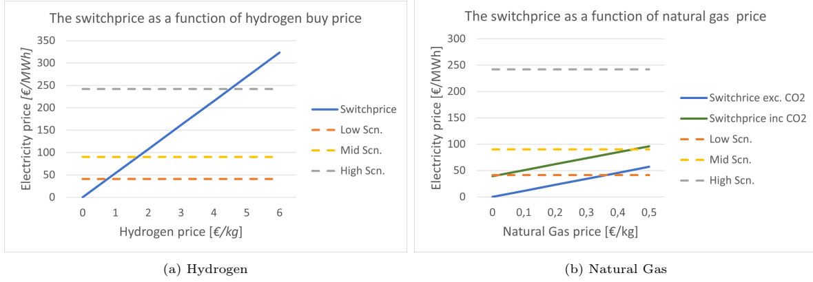
Figure 4.18: Back of the envelope relation of secondary feedstock prices to the switch-price, using Equation 4.1, to point out the advantage of natural gas due to switch-price. power price scenario levels are plotted for reference. Total system efficiency \eta_{FC,H_2,LHV}=50\% , \eta_{FC,H_2,LHV}=60\% , \theta_{CO_2,buy}=125 €/tonne , f_{HS}=5\%
