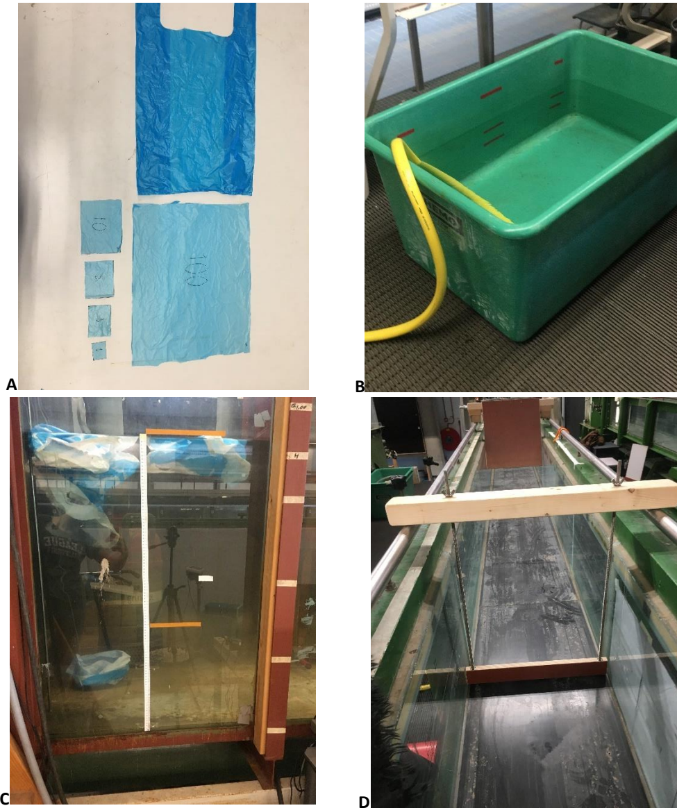
Fig. 20: A: HDPE bag and different sizes of sheets, B: the container used for rise velocity experiments with different scales, C: the tank used for the rise velocity experiments with bags and foils, D: an obstruction placed in the flume. In this scenario it is a bottom sill (5 cm).
