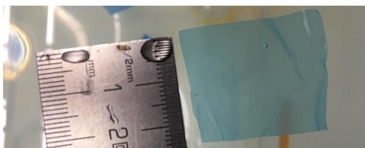
Figure 4.5: Image showing the presence of air-bubbles on the plastic, with a diameter of about 1 mm
