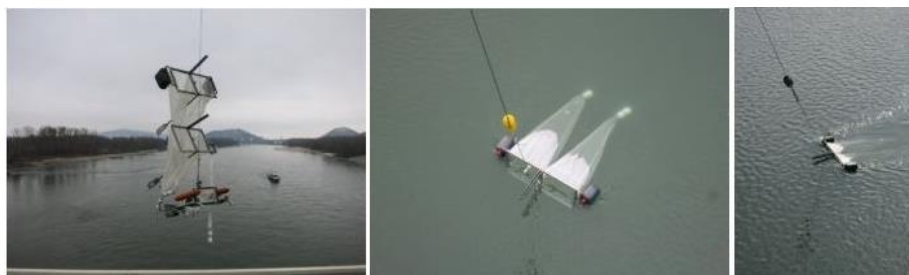
Figure 1.2: Triple-layered sampling net used for a study in the Danube (Hohenblum et al., 2015).
