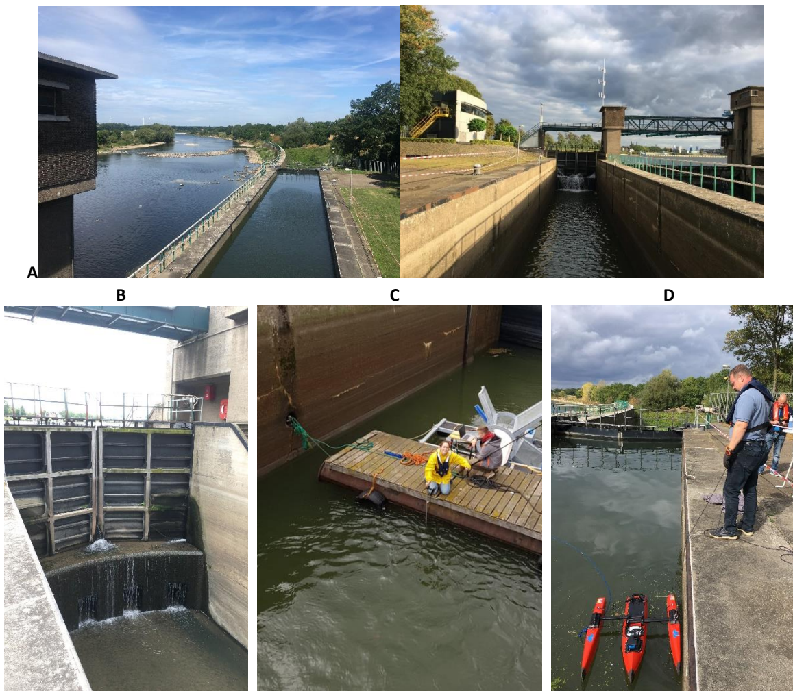
Fig. 24: Impression of Borghare Sluice measurements. A: sluice next to Grensmaas, B: inlet doors and inlet sewers below, C: flow measurements with ADP flow meter, D: flow measurements with ADCP catamaran, executed by RWS.
