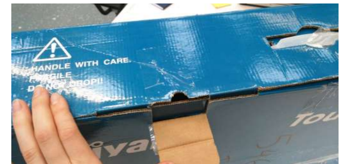
Figure A.39 Tuck top with reverse tuck flap in existing packaging (tuck flap pulled back)
