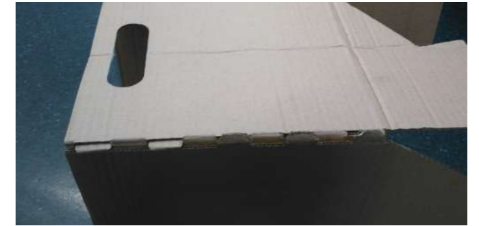
Figure A.37 First form fit closure, comparable to small waste bin
