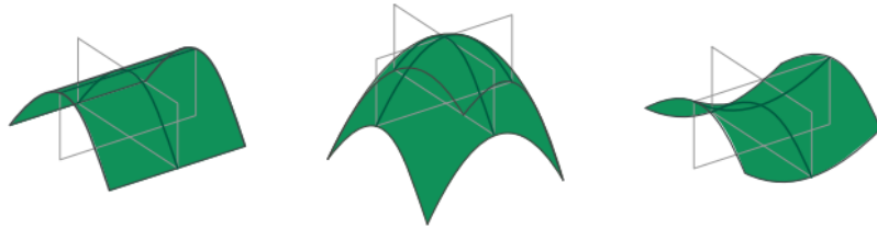
Figure 2.2: Possible types of double curvature, from left to right: monoclastic, synclastic and anticlastic[9]
