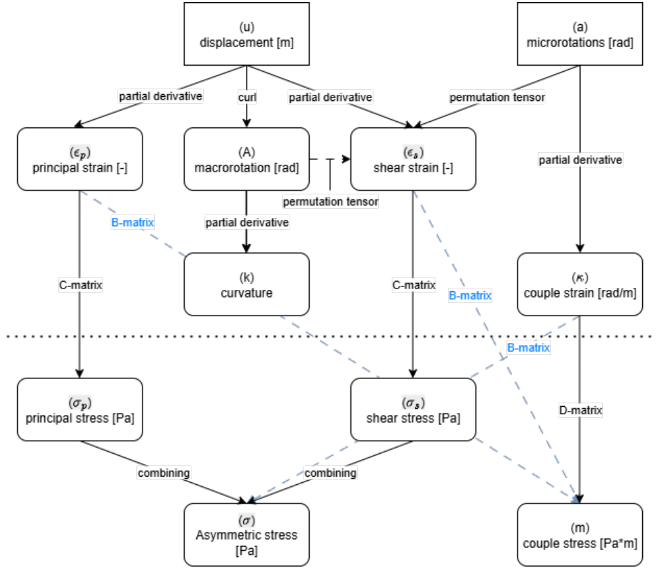
Figure 2.8: visualisation of how the global variables (translations and microrotations) are related to the derived variables
