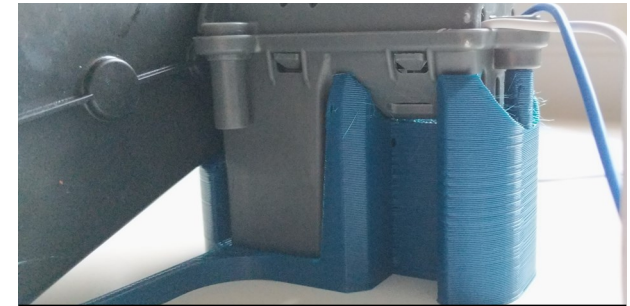
Figure 21.1: Early test of a 3D printed motor mount
