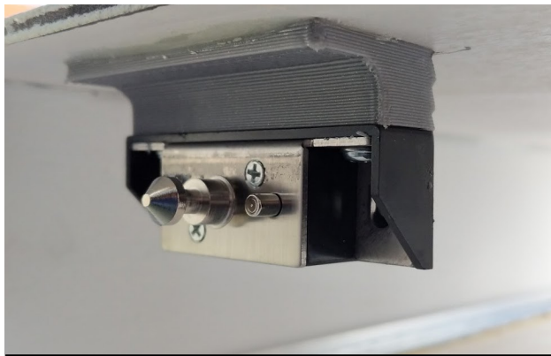
Figure 21.14: Locking pin attached to the modular container
