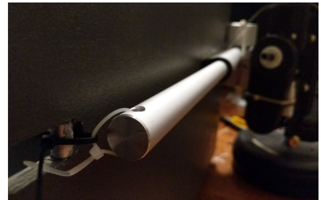
Figure 21.13: 200N linear actuator (photo taken from the top)
