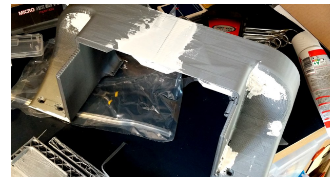
Figure 21.8: Plastered plastic rear part with wheel arches
