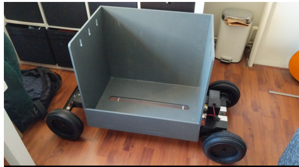
Figure 21.5: Core module placed on the chassis
