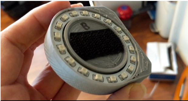
Figure 21.19: 3D printed LED-ring holder with Velcro
