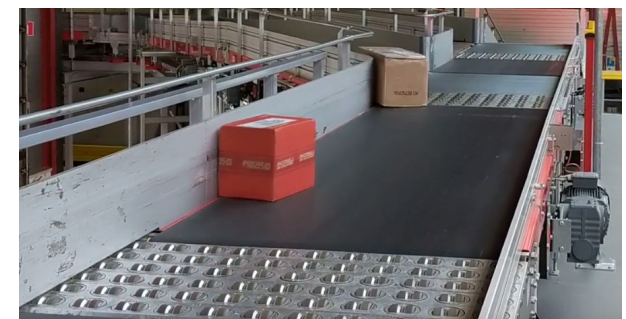
Figure 17.3: The 'wheels' guide the brown box to the left
