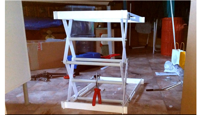
Figure 21.12: Working scissors mechanism
