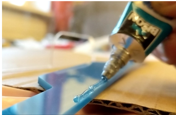
Figure 21.15: Gluing the acrylic
