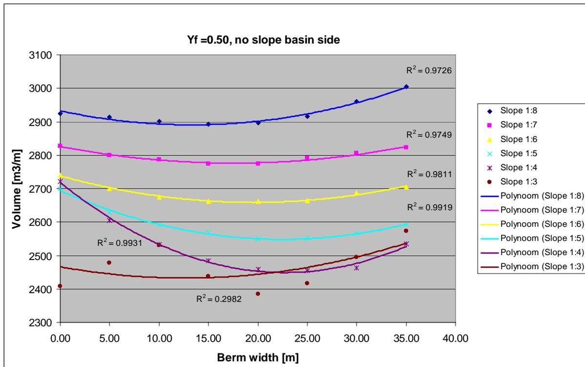
Figure 64: volume as a function of the outer berm width, surface roughness factor is 0.50.
