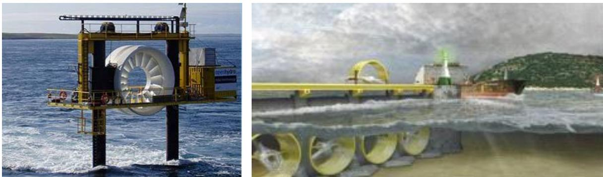
**Figure 70:** on the left a tidal stream turbine (Courtesy: *OpenHydro*), on the right an artist impression of the Severn tidal fence (Courtesy: *unknown internet source*).
