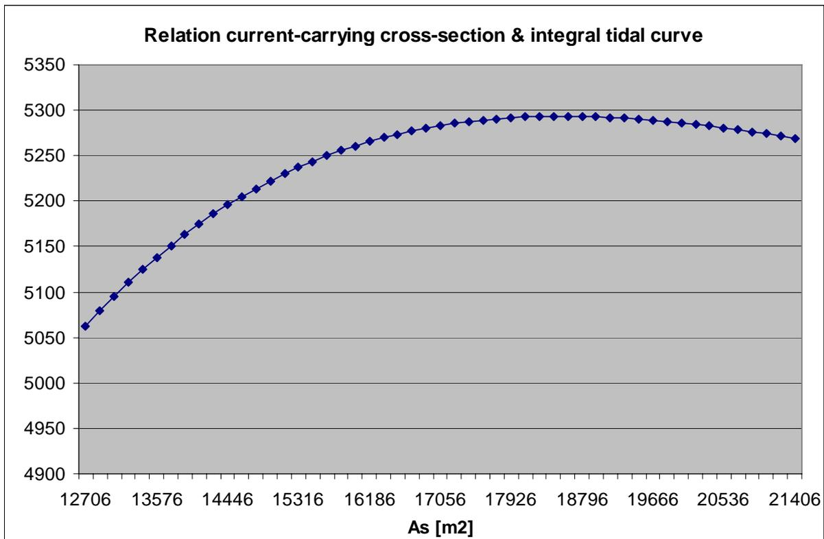
Figure 90: relation current-carrying cross-section and the area under the tidal curve.
