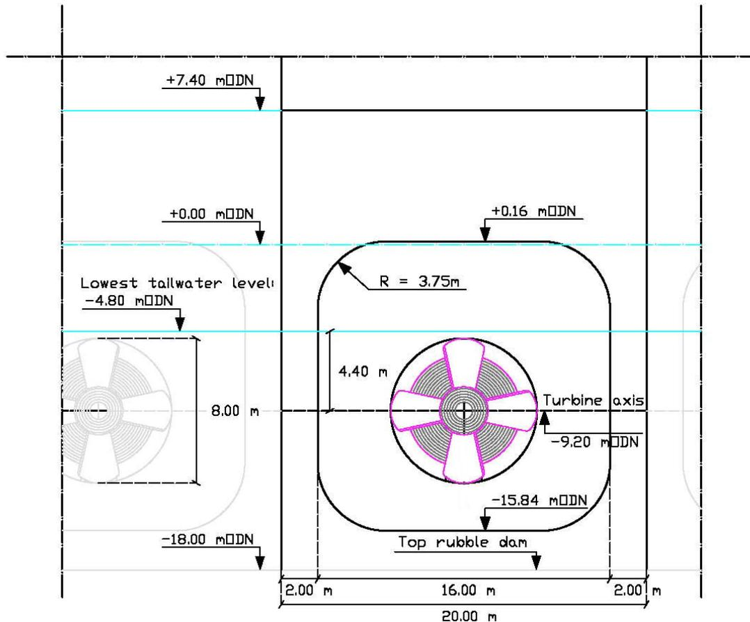
Figure 83: front view turbine caisson (not to scale).
