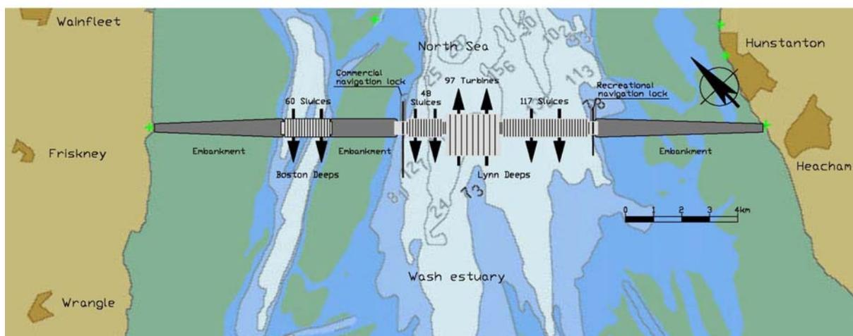
**Figure 96:** bird-eye view of the Wash estuary storm surge barrier and tidal power plant.
