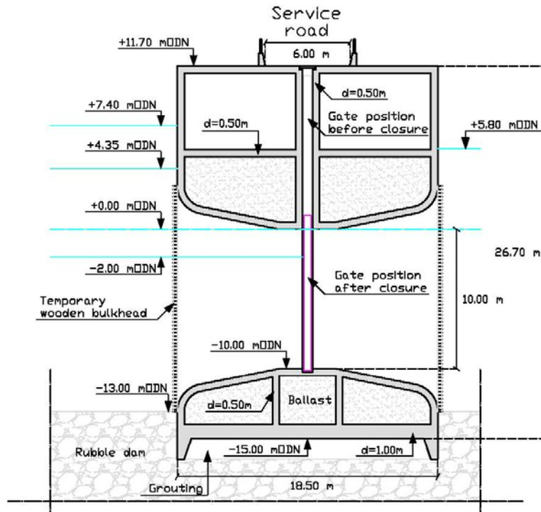
Figure 87: front view sluiced caisson Lynn Deeps (not to scale).
