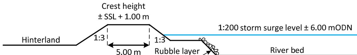
Figure 30: average cross-section of the river defences bordering the tidal rivers.
