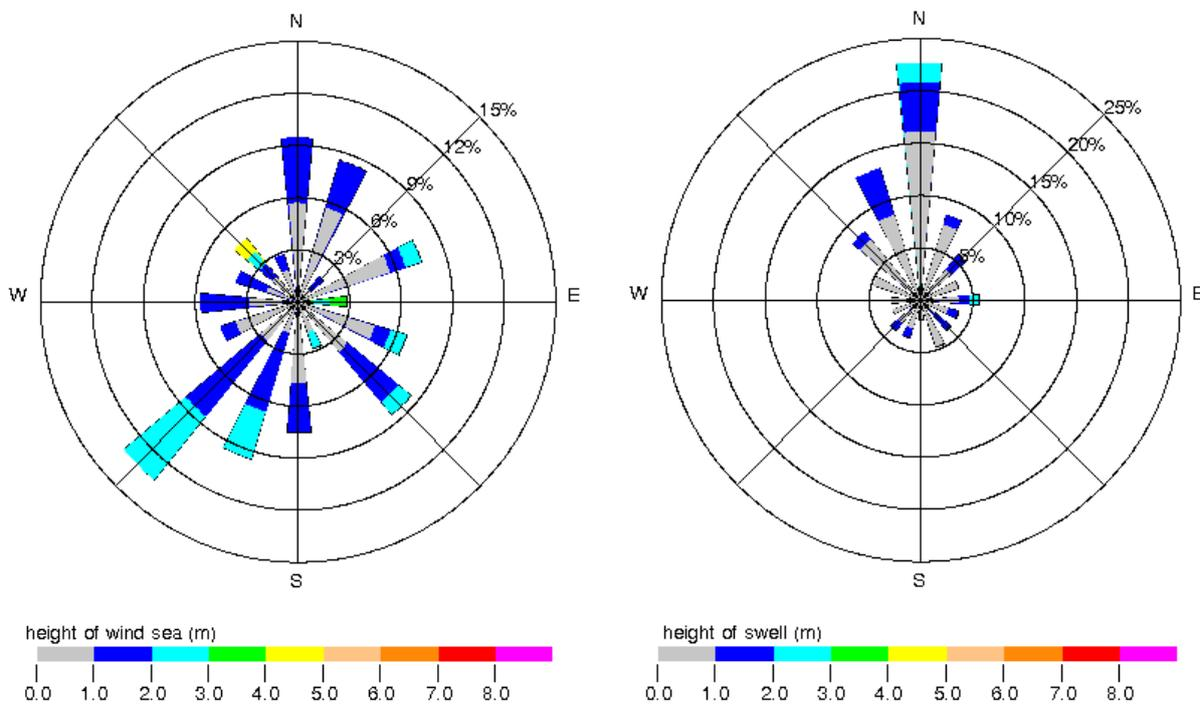
Figure 38: on the left: wave height rose regarding wind sea. On the right: wave height rose regarding swell (Courtesy: BMT ARGOSS).
