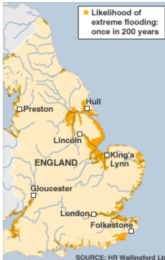
**Figure 43:** area flooded during a 1:200 yr storm surge in absence of flood defences.
