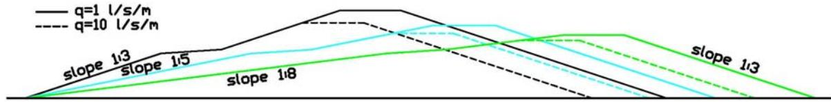
Figure 59: relation crest height and overtopping discharge.
