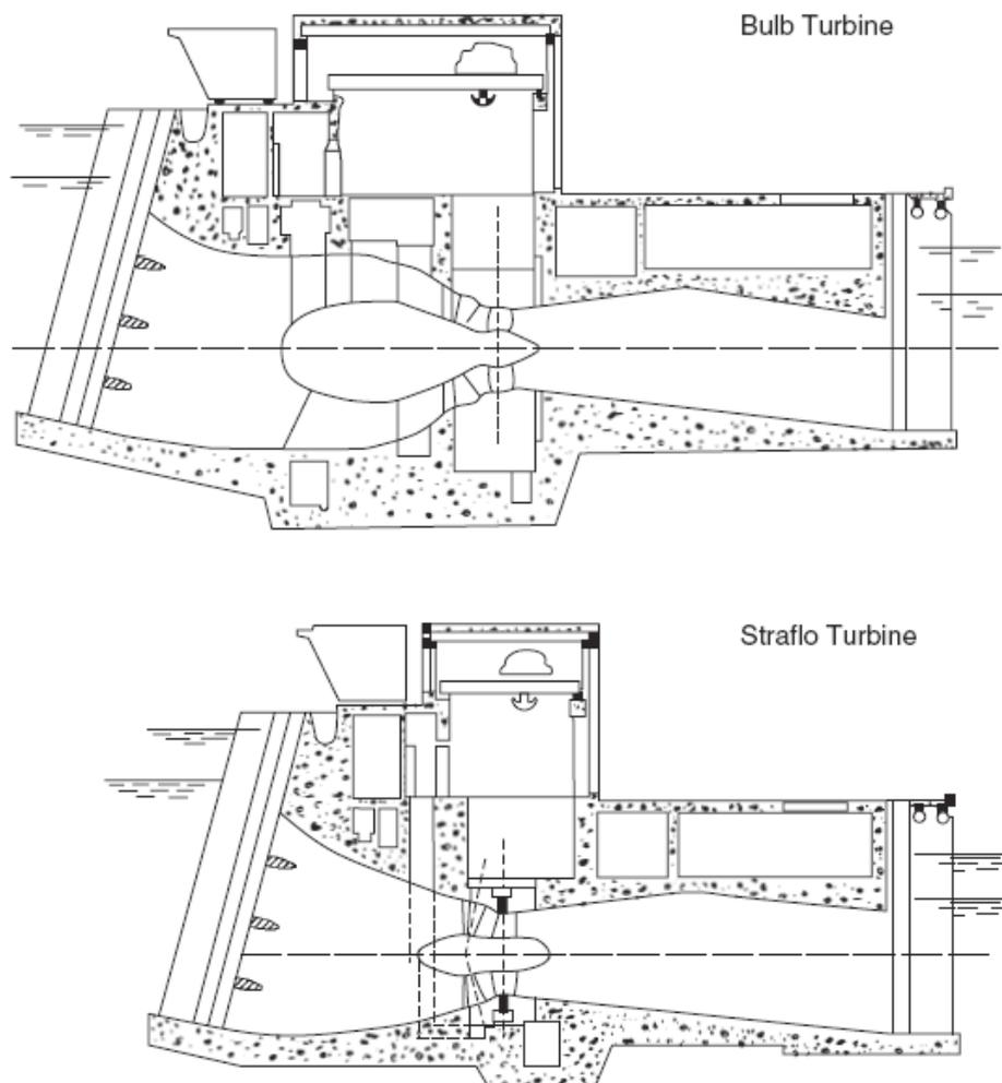
**Figure 72:** comparison of straflo and bulb turbine powerhouses for the same output and head.
