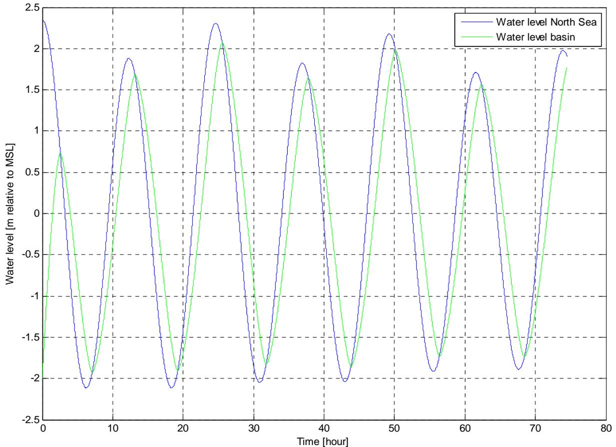
Figure 91: impact of the final conceptual design on the amplitude of the water level within the basin.
