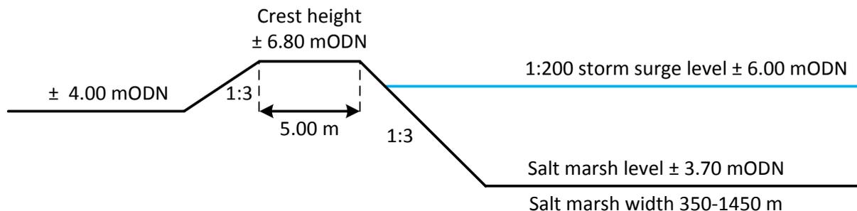
Figure 53: average cross-section of the flood defences bordering the Wash estuary.
