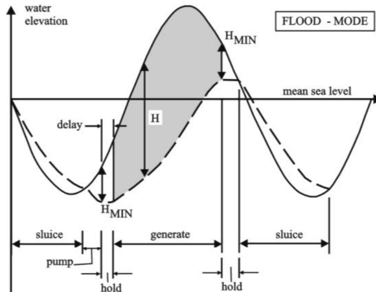
Figure 77: water level versus time during flood generation (Courtesy: Wyre tidal energy).
