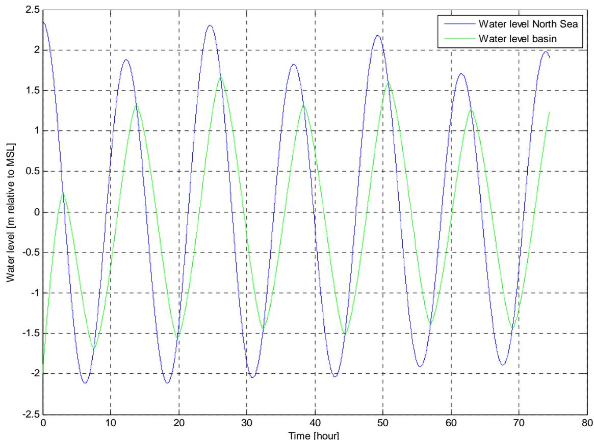
**Figure 89:** impact of the preliminary design on the amplitude of the water level within the basin.
