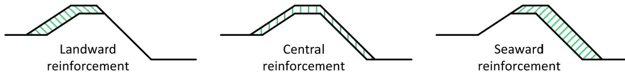
Figure 54: landward, seaward and central reinforcement.
