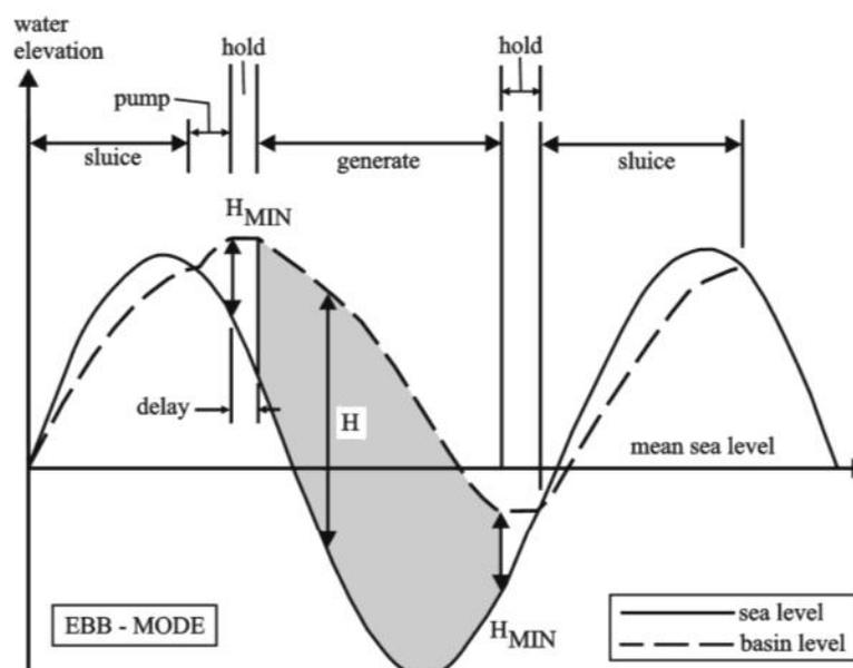
Figure 76: water level versus time during ebb generation (Courtesy: Wyre tidal energy).
