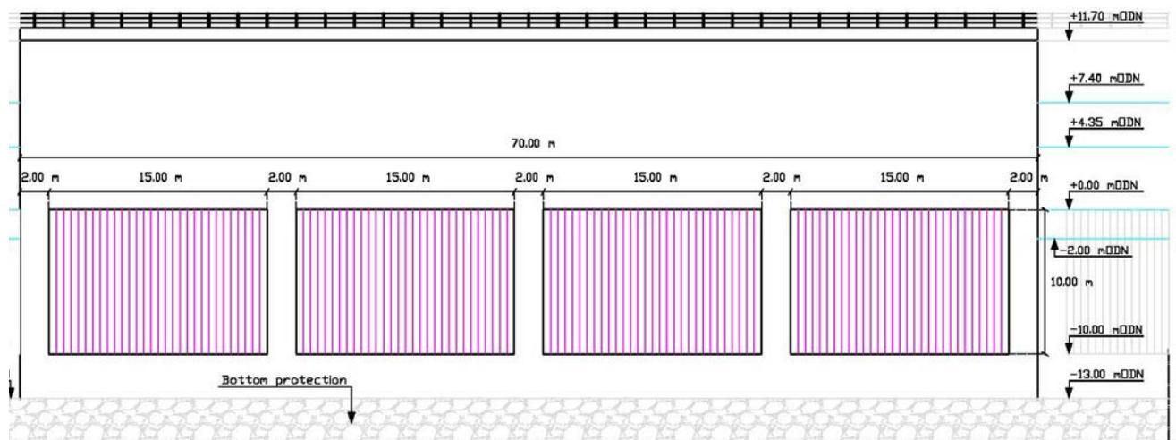
Figure 86: front view sluiced caisson Lynn Deeps (not to scale).
