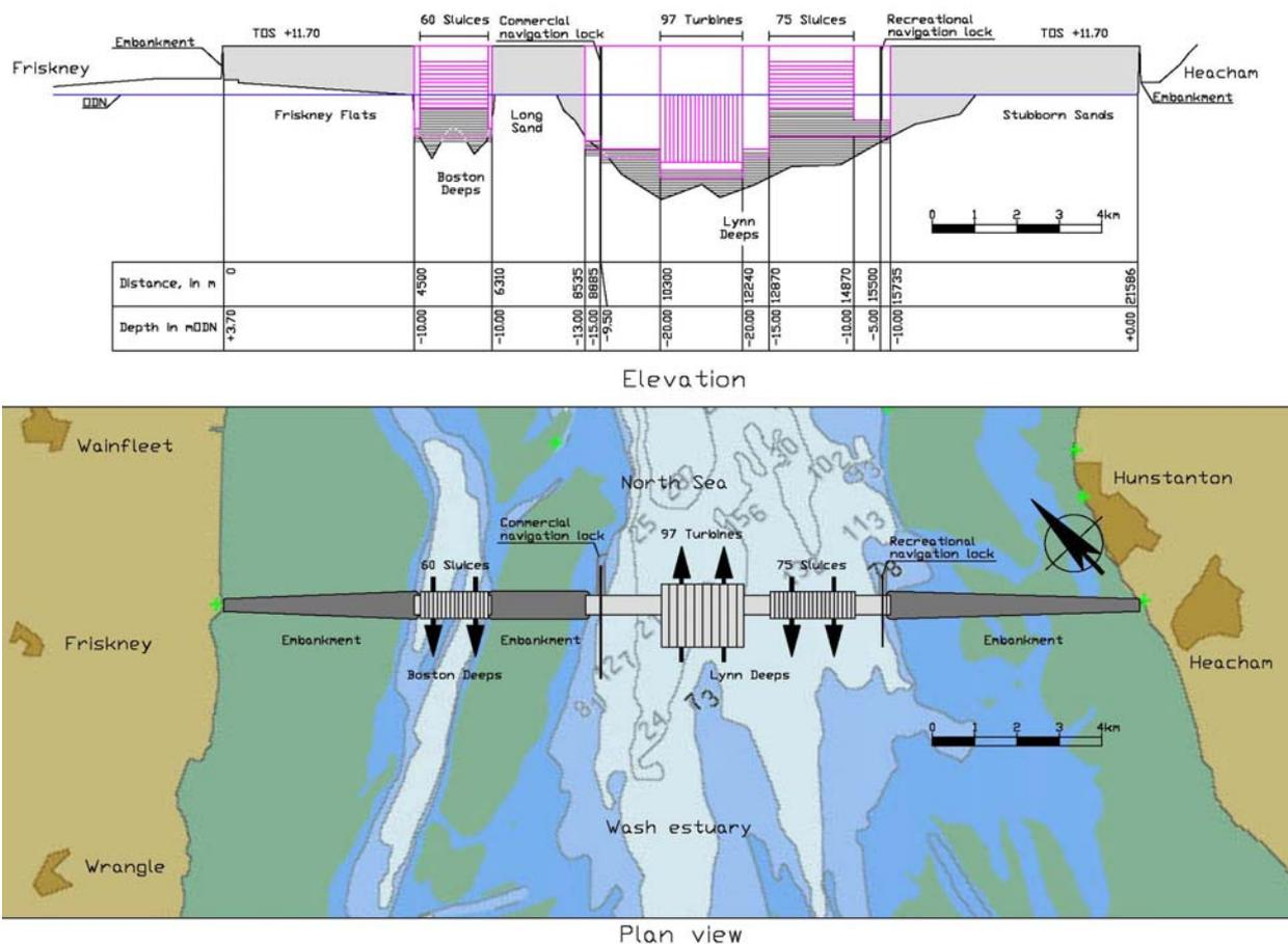
Figure 88: preliminary design of the combined storm surge barrier and tidal power plant in the Wash estuary.
