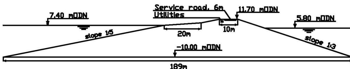
Figure 65: preliminary cross-section permanent barrier (not to scale).
