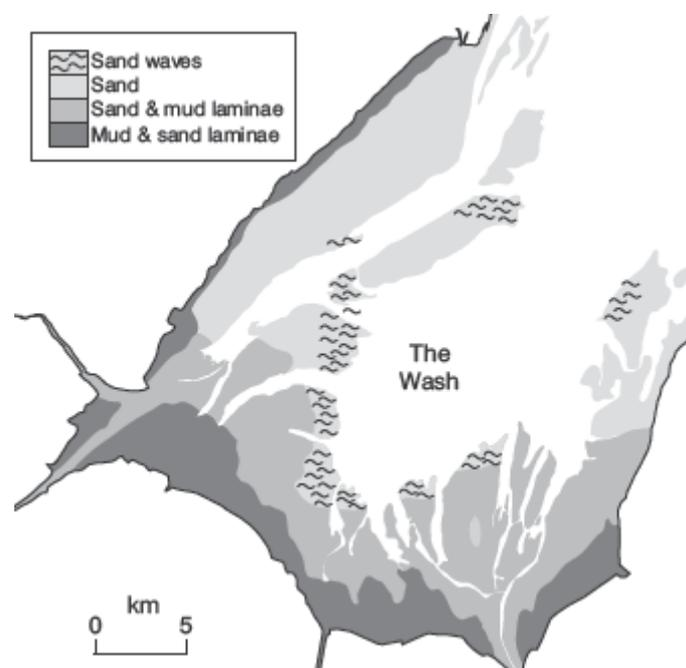
**Figure 37:** distribution of intertidal sediments in the Wash.
