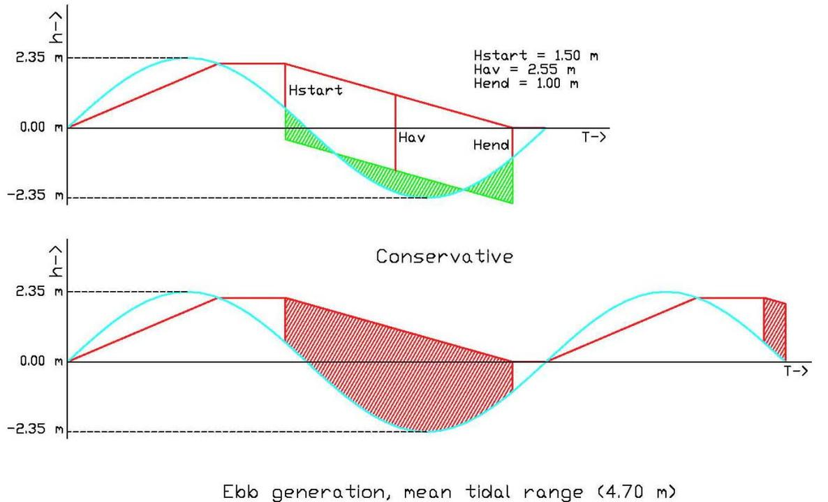
**Figure 80:** schematic representation of TPP operation in case of an ebb generation scheme (not to scale).
