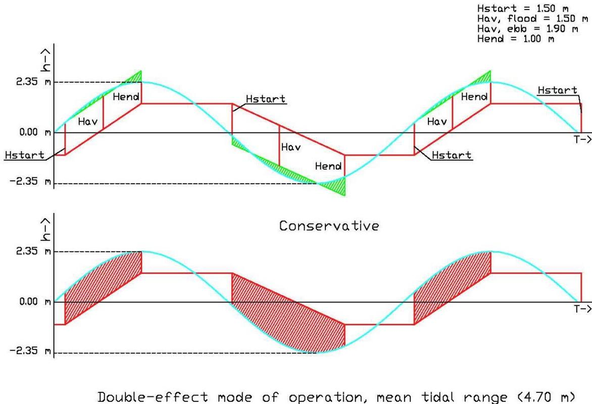
**Figure 81:** schematic representation of TPP operation in case of a two-way generation scheme (not to scale).
