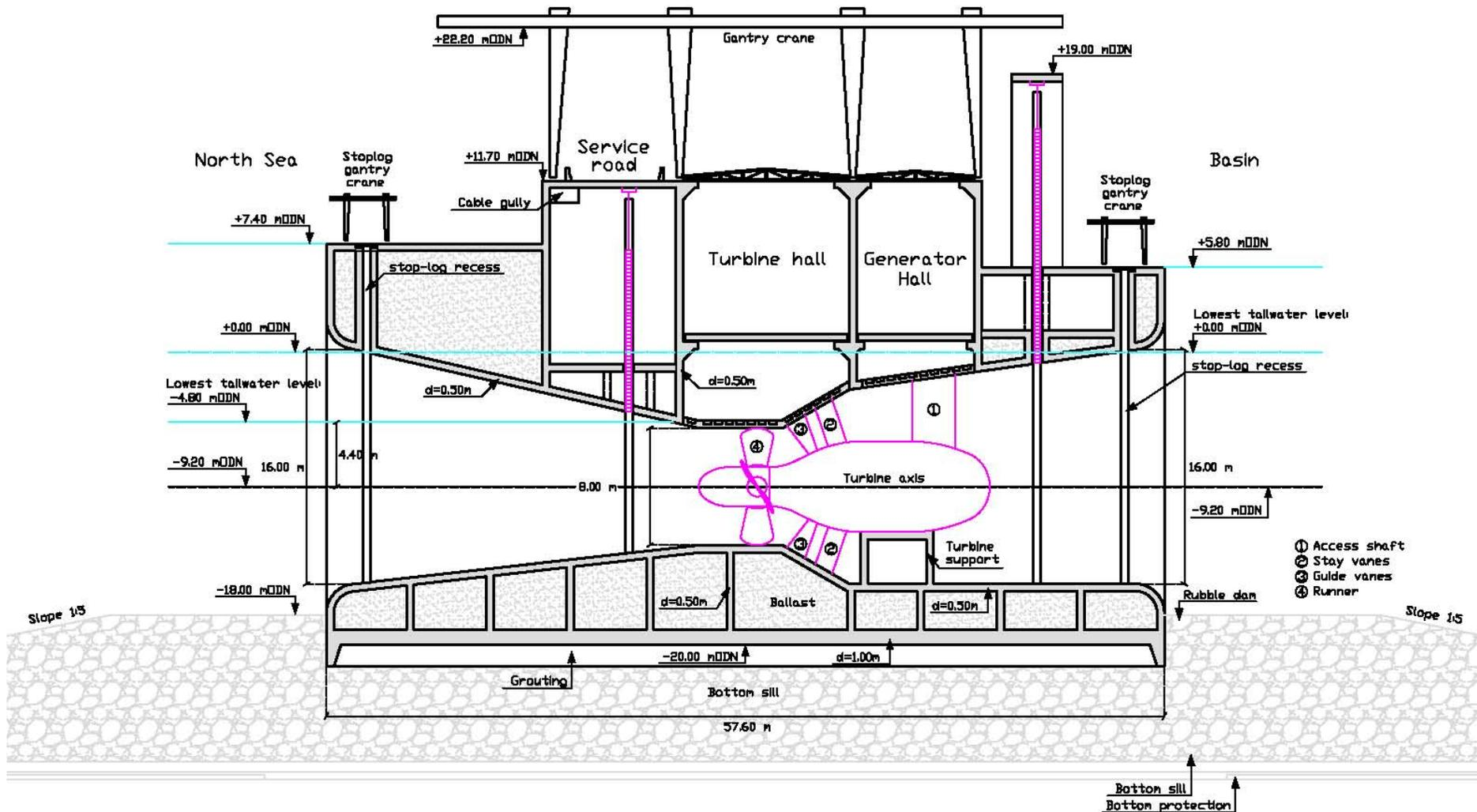
Figure 82: cross-section turbine caisson (not to scale).
