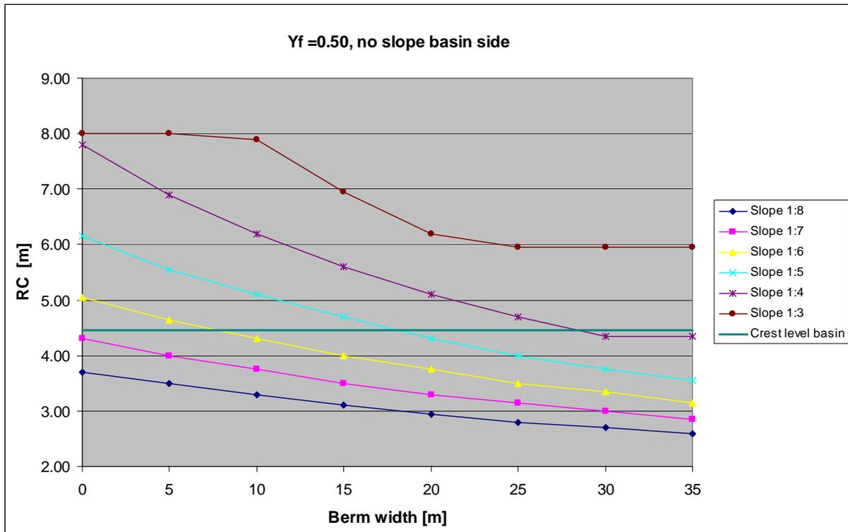
Figure 62: crest height above SWL as a function of the outer berm width, surface roughness factor is 0.50.
