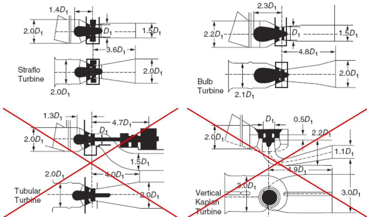
Figure 71: overall dimensions for low-head turbine designs (Courtesy: Clark, 2007).
