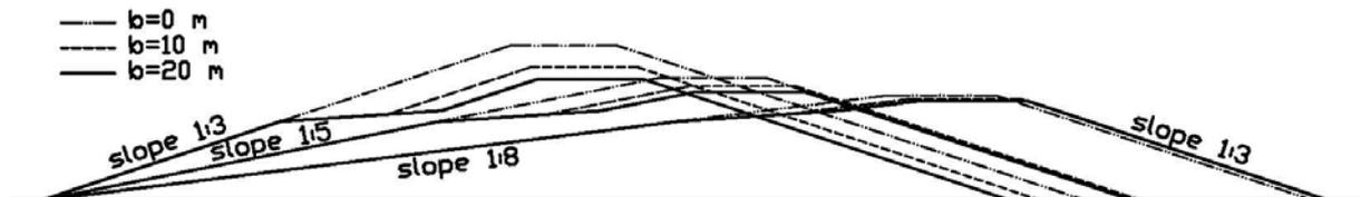
Figure 63: relation crest height and berm width.
