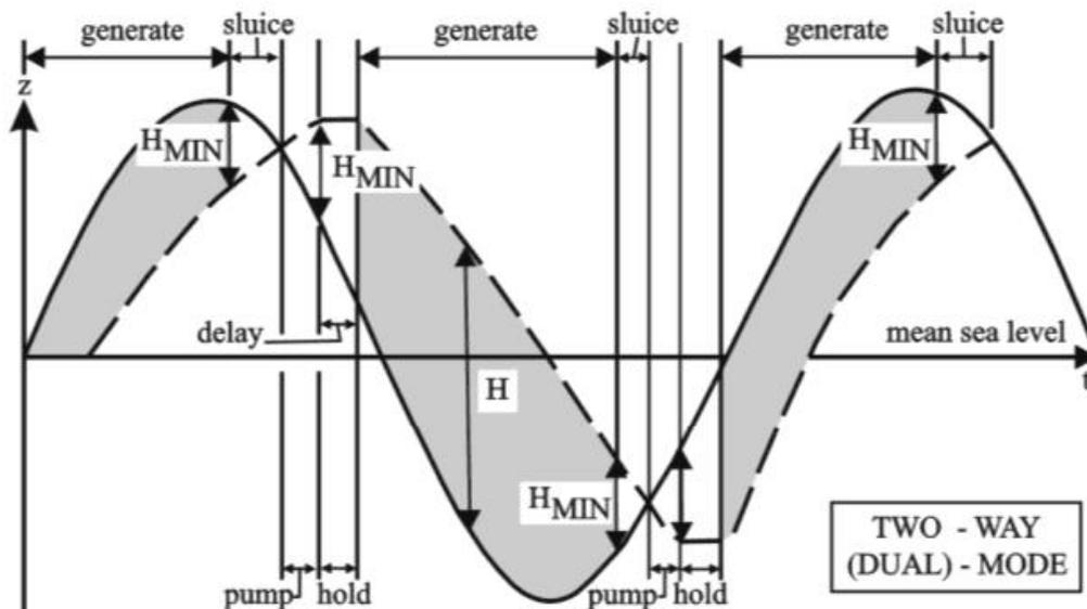
Figure 78: water level versus time during double-effect operation (Courtesy: Wyre tidal energy).
