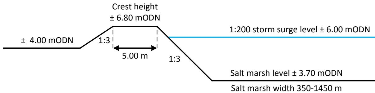
Figure 28: average cross-section of the flood defences bordering the Wash estuary.
