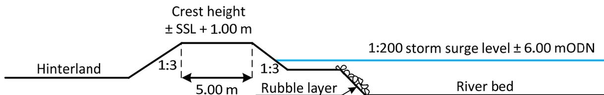
Figure 56: average cross-section of the river defences bordering the tidal rivers.
