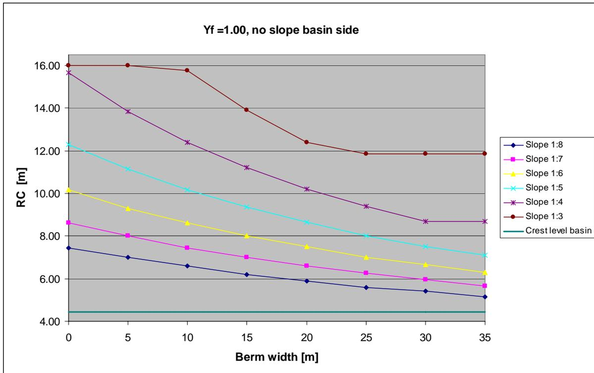
Figure 61: crest height above SWL as a function of the outer berm width, surface roughness factor is 1.00.
