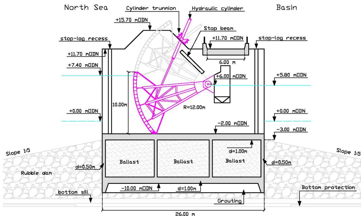
Figure 84: cross-section sluice gate configuration (not to scale).
