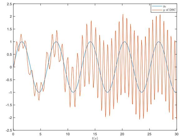
Fig. 4. System output  $y$  of DSC and desired signal  $y_d$  with  $\tau_2 = 0.2$
