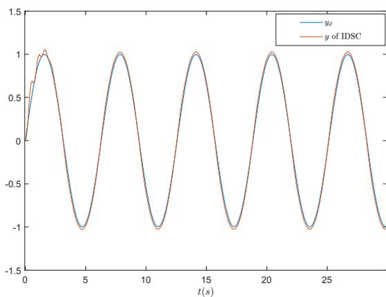
Fig. 7. System output  $y$  of IDSC and desired signal  $y_d$  with  $\tau_2 = 0.2$
