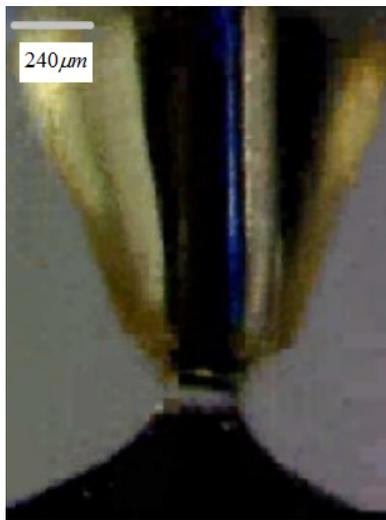
**Figure 3-3:** The last frame before the liquid bridge breaks.
