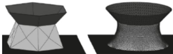
**Figure 1-13:** Shape of the Liquid bridge between a conical tip and a surface: the left one is before optimization and the right is after optimization using "surface evolver" [21].
