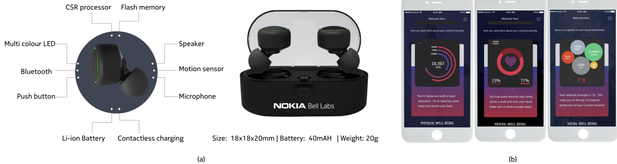
Figure 1: (a) eSense open wearable platform with audio, motion, and BLE sensing powered by a CSR processor and a 40mAH battery and (b) eSense manifested in a well-being feedback application in a quantified enterprise environment
