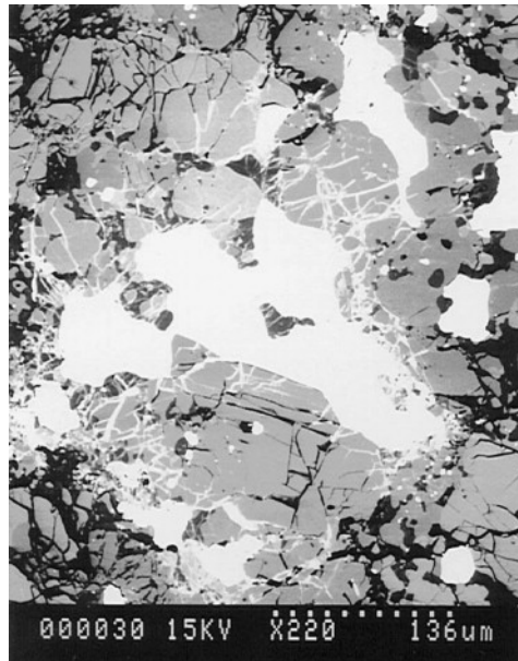
Figure 3.6: Slice image of an H5 ordinary chondrite. The black veins show the cracks accounting for the microporosity. The white areas show grains of Iron and Nickel. The partial filling of the microcracks with white material is thought to be the result of oxidation of the metallic grains with terrestrial Oxygen. From "The significance of meteorite density and porosity", by G.J. Consolmagno et al. [53].
