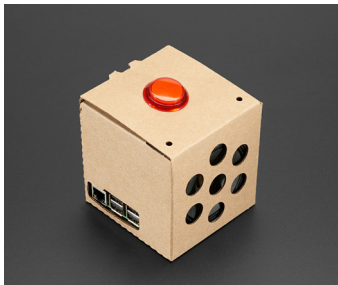
AIY voice kit to prototype voice assistant interface using Natural Language Processor
