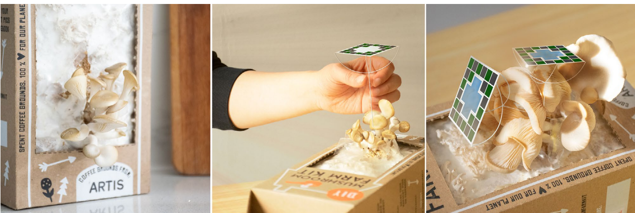
Figure 4.16.: Mushroom Shade: Under excessive sunlight, the EC unit of the interface would darken its colour, casting a protective shadow onto the fungi body underneath. Users can provide care to the mushrooms in a delicate way, by “planting” the Mushroom Shade above each cluster of fruiting bodies.
