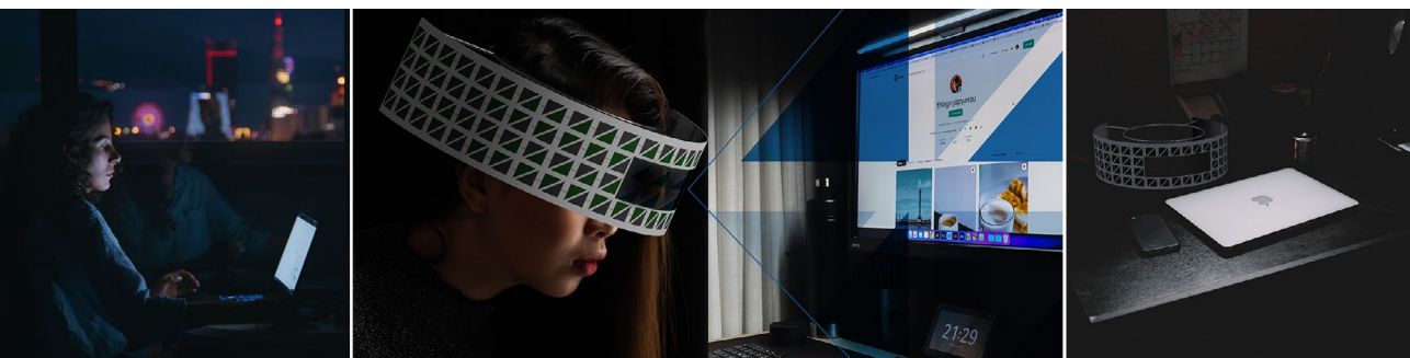
Figure 4.15.: Circadian Navigator: As the cyano unit of the artefact reacts to the light emitted from the screen, the EC component would darken its colour which would subsequently restrict the opacity of the worn lenses (i.e., visibility), nudging the wearer away from their screen use.
