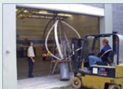
A Darrieus turbine is being transported to the wind tunnel of the Wind Energy section at TU Delft to be tested for the Eneco power company.
