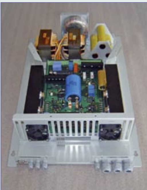
Since Turby is not self-starting Sidler developed a 'dedicated' converter. It is a four-quadrant system, which handles not only the start-up function of the synchronous generator as a drive motor, but also the turbine control and safety functions and the conversion of the variable voltage and frequency generated by the generator to the correct voltage and frequency so the wind-generated electrical power can be fed into the local grid.
