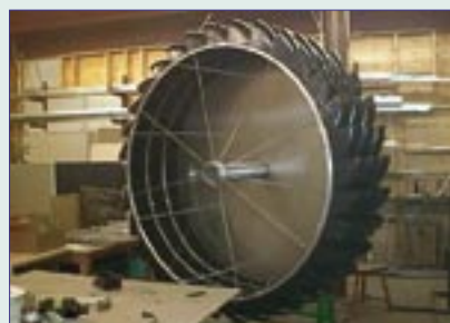
The drum-shaped rotor of the Catavent wind turbine showing the vanes fitted to the outside of the drum.
