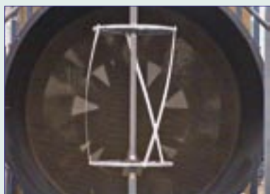
The first prototype Turby in front of the wind tunnel of the Wind Energy section at TU Delft's Stevin Laboratory. It has racing bike wheels fitted with aerodynamic spokes at its top and bottom. The manufacturer of the first prototype thought the aerodynamic spokes would keep the drag figure down. However, the model disintegrated because the bolt used to secure the position of the two wheels broke
