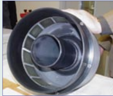
Interior view of the rotor with permanent magnets. These magnets have been fitted at a slight angle in order to reduce the adhesion forces that would hold the rotor in a preferred position, requiring an extra force to set the rotor in motion.
