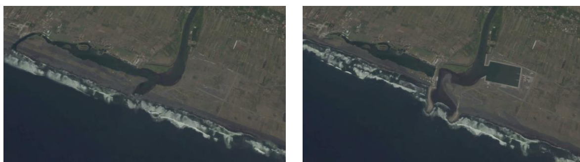
FIGURE 2-8 COASTLINE BEFORE AND AFTER CONSTRUCTION OF THE BREAKWATERS (ESTIMATION)
