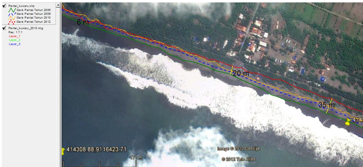
FIGURE 2-10 COASTLINE RETREAT AT KAWURA BEACH (12 KM EAST OF THE GLAGAH JETTY PROJECT SITE)
