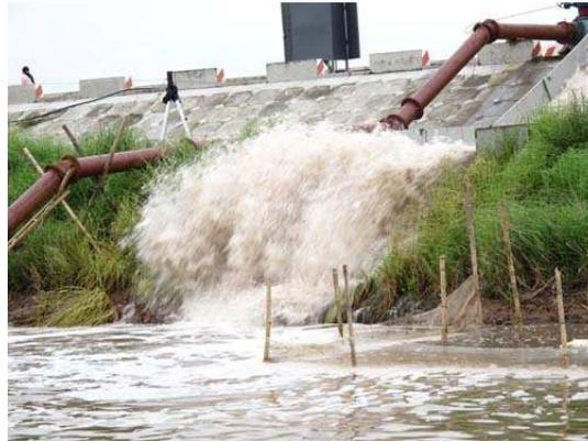
Figure 12. Flow flying from the inner berm attacked the dike toe.
