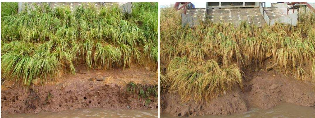
Figure 18. Vetiver grass slope at location DS\_01. Left: after 4 hours of 20 l/s per m and 1 hour of 40 l/s per s. Right: final situation.
