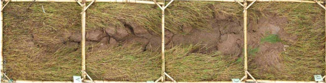
Figure 9. Damage on the Bermuda grass slope with rectangular shape.
