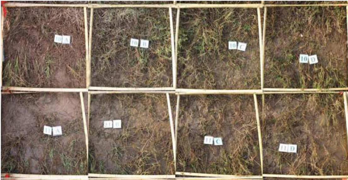
Figure 10. Poor coverage of grass at the transition between the dike slope and the dike foreland.
