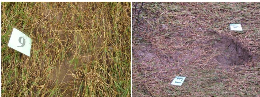
Figure 8. Left: single damage hole after 4 hours of 10 l/s per m and 2 hours of 20 l/s per m. Right: 2 hours extra of 20 l/s per m, tendency of combining two separate holes close to each other.
