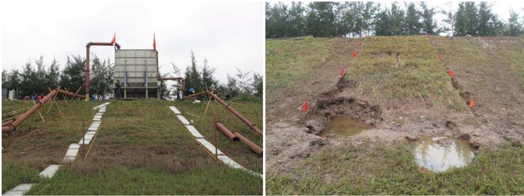
Figure 14. Grass slopes at test location TL\_01: initial situation (left) and final result (right).
