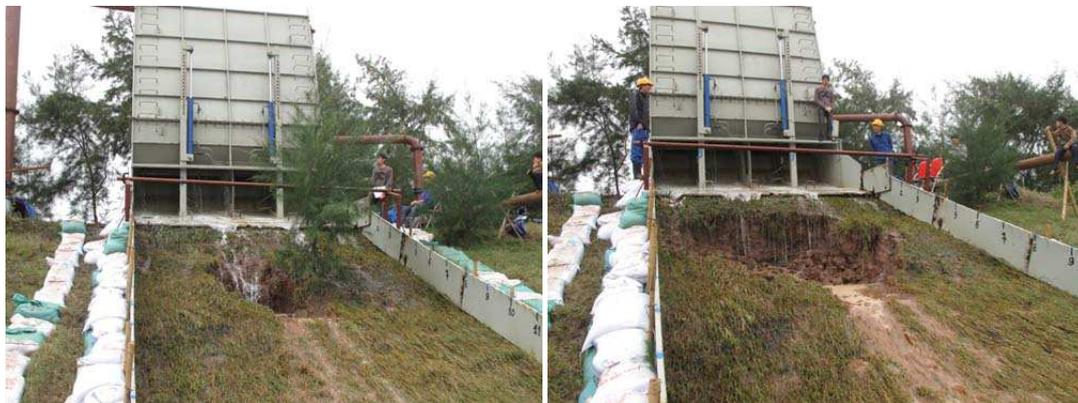
Figure 7. Dike slope after 4 hours of 10 l/s per m (left) and after that 30 minutes of 20 l/s per m, the 7-cm-diameter casuarina collapsed (right).
