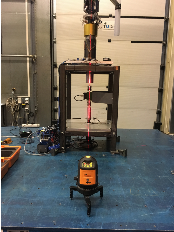
Figure 6: Gadella FL 55 Plus laser alignment system is used to align the azimuth position and pitch position of the PitchVAWT turbine to the Open Jet Facility tunnel outlet.
