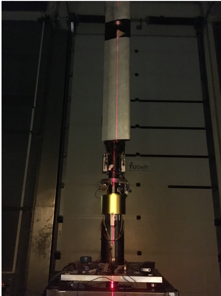
Figure 8: Alignment laser setup for zeroing turbine azimuth position
