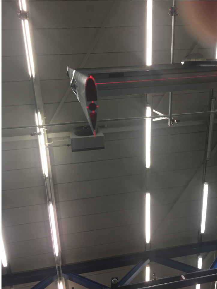
Figure 10: Alignment laser for setting pitch
