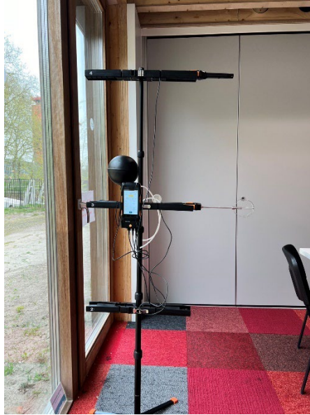
Figure 29: The setup of Testo 400 with other sensors on a tripod.
