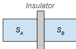
Figure 2.1: Simple schematic of a Josephson junction.
