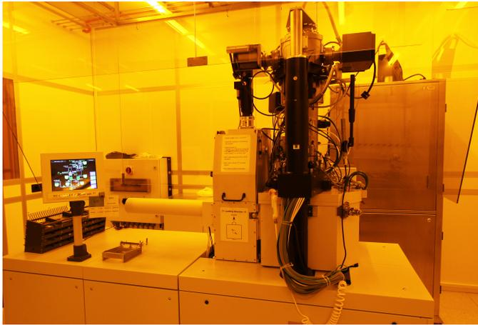
Figure 3.4: The setup used showing the Raith EBPG-5000+, picture from [31].
