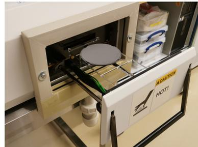
(b) A picture showing how samples are loaded.
