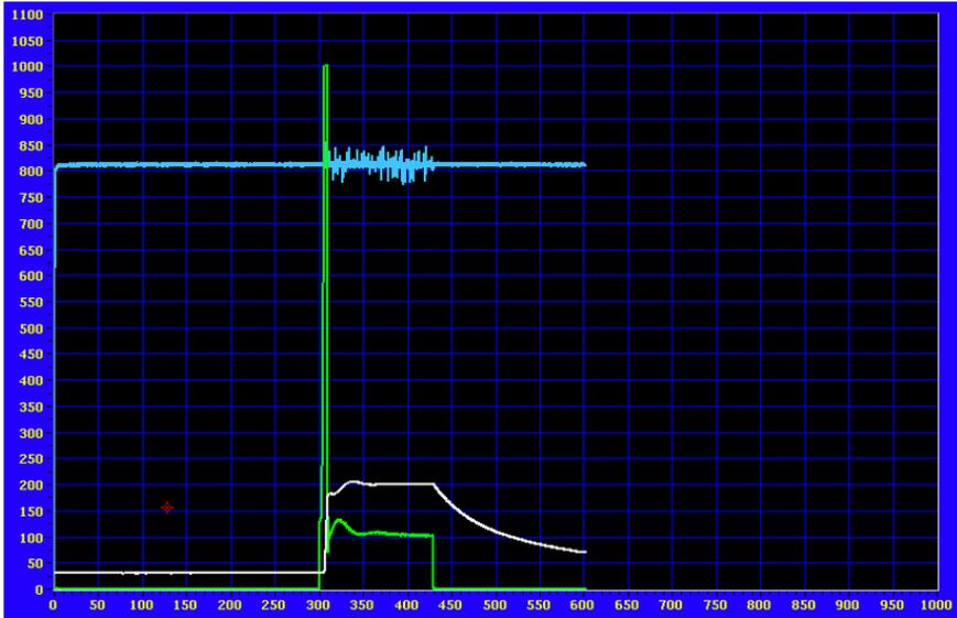
Figure 3.17: Graph showing the control temperature, total flow, and power input over time in the colours white, blue and green respectively. The process shown here was a typical 200°C anneal using forming gas (90% N<sub>2</sub> / 10% H<sub>2</sub>).
