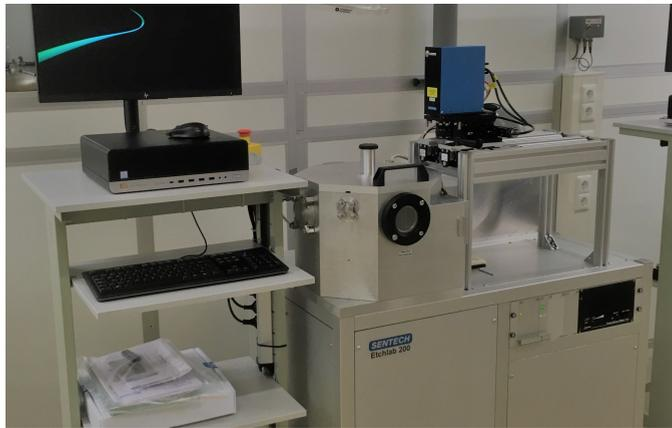
Figure 3.6: The setup used showing the Sentech Etchlab 200, picture from [31].
