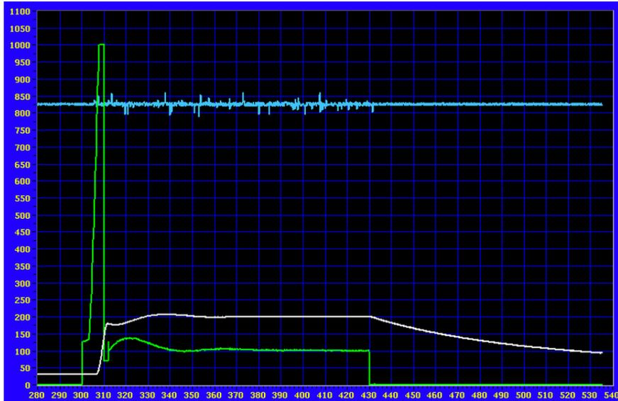
Figure 3.14: Graph showing the control temperature, total flow, and power input over time in the colours white, blue and green respectively. The process shown here was a typical 200°C anneal using N<sub>2</sub>.
