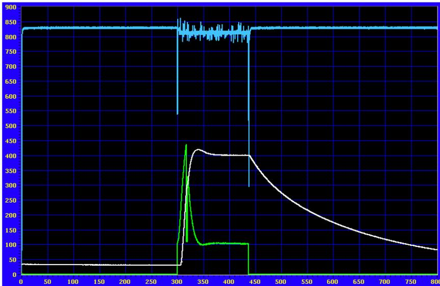
Figure 3.19: Graph showing the control temperature, total flow, and power input over time in the colours white, blue and green respectively. The process shown here was a typical 400°C anneal using forming gas (90% N<sub>2</sub>/ 10% H<sub>2</sub>).
