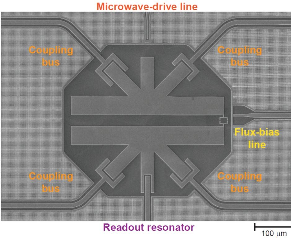
Figure 2.7: Starmon device, the red, orange, yellow and purple labels show the Microwave-drive line, coupling busses, flux-bias line and readout resonator respectively. Image from [24, p. 7].
