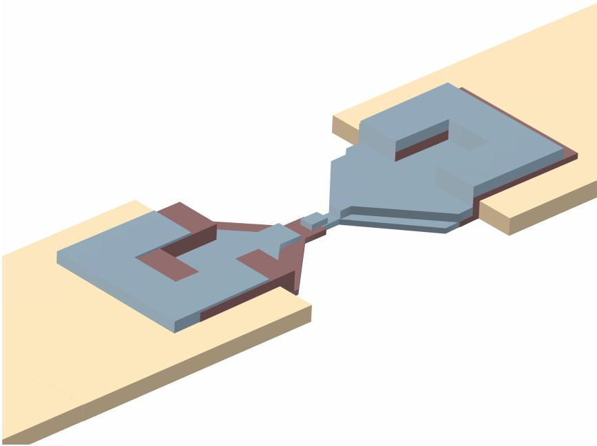
Figure 2.5: A Dolan type Josephson junction which is formed using a shadow evaporation technique. The yellow colour indicates the contacts, the first deposited layer of metal is red, the second layer which is deposited with a  $180^\circ$  rotation is coloured blue. Due to the shadowing technique the layers overlap at multiple places not just at the junction in the middle.
