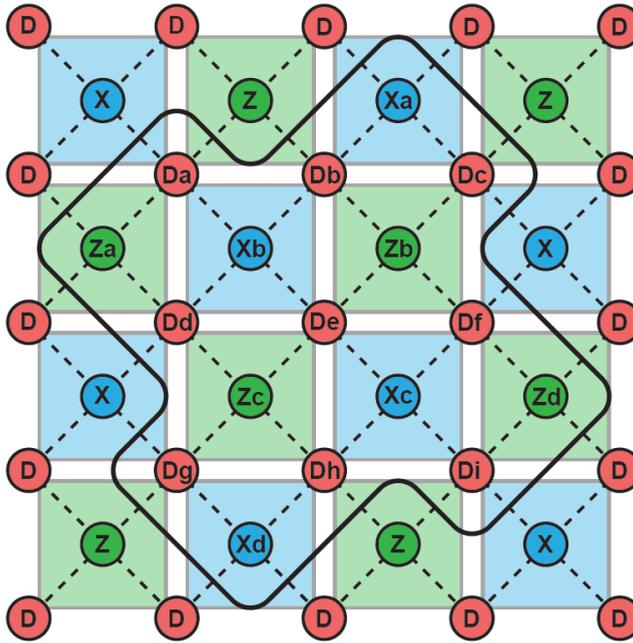
Figure 2.8: Surface-code fabric design, the red circles indicate data qubits, the blue and green circles indicate ancilla qubits which are used for error correction. The black boundary line surrounds a distance-3 planar logical qubit which is named Surface-17. Image from [24, p. 2]
