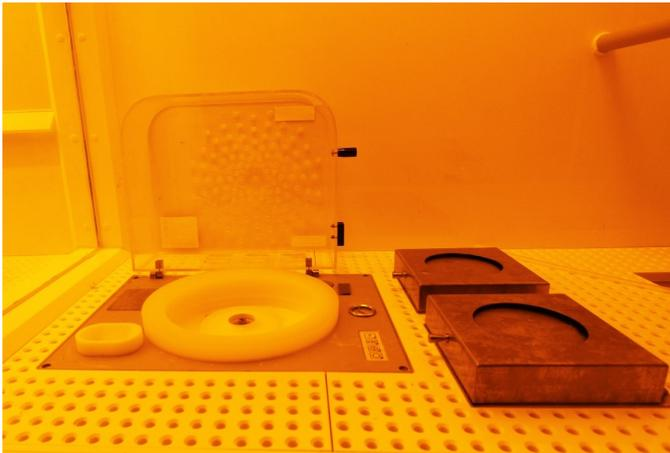
Figure 3.3: The setup used showing the spin coater and hotplate, picture from [31].
