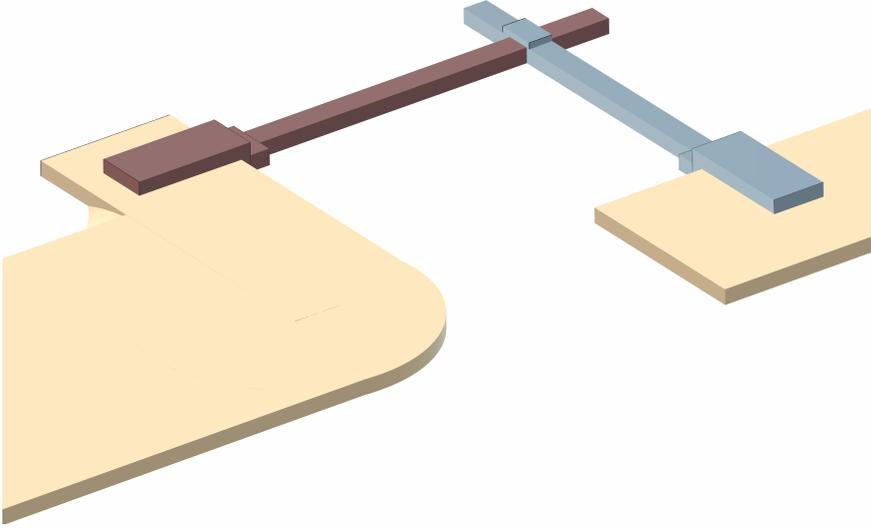
Figure 2.6: A Manhattan type Josephson junction which is formed using a top-heavy resist stack. The yellow colour indicates the contacts, the first deposited layer of metal is red, the second layer which is deposited with a  $90^\circ$  rotation is coloured blue. To make sure that there is a proper connection between the electrodes and the contacts the metal layers are deposited aiming towards the contacts. Because of this angle there is a slight shadowing effect near the junction.
