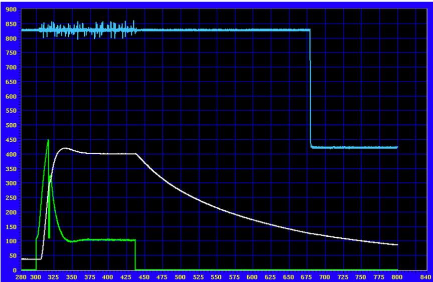
Figure 3.16: Graph showing the control temperature, total flow, and power input over time in the colours white, blue and green respectively. The process shown here was a typical 400°C anneal using N<sub>2</sub>. In this recipe the setpoint is also overshoot as can be seen at  $t \approx 340$  s.
