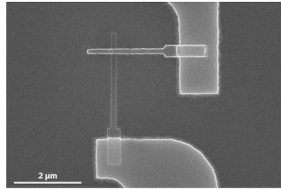
(b) The two overlapping electrodes of a Manhattan type JJ
