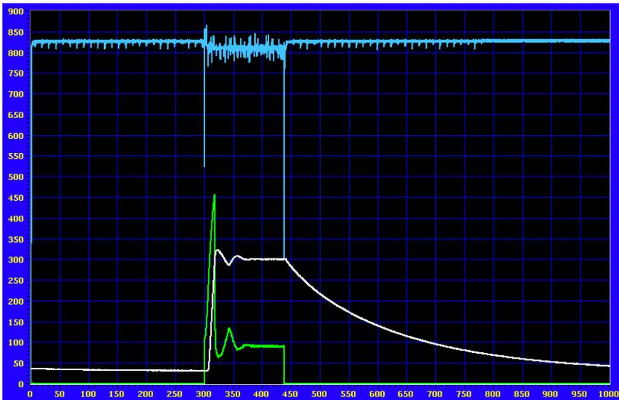
Figure 3.18: Graph showing the control temperature, total flow, and power input over time in the colours white, blue and green respectively. The process shown here was a typical 300°C anneal using forming gas (90% N<sub>2</sub> / 10% H<sub>2</sub>). From  $t \approx 310$  s to  $t \approx 360$  s there is some overshooting, and the system overreacts making it take a bit longer to reach a stable 300°.
