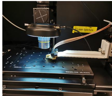
(b) A die loaded on the horizontal XY-stage of the APS.
