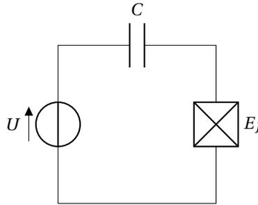
Figure 2.2: Charge qubit circuit.
