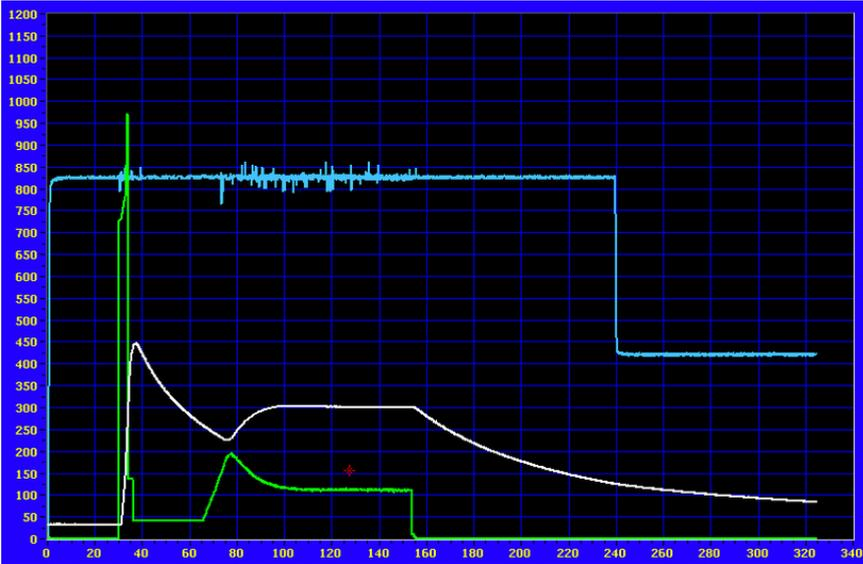
Figure 3.15: Graph showing the control temperature, total flow, and power input over time in the colours white, blue and green respectively. The process shown here was a typical 300°C anneal using N<sub>2</sub>. Notice the initial spike here around  $t \approx 40$  s, it shows that the temperatures overshoot the setpoint of 300°C by a lot. After this the temperature drops down to below 250° and as can be seen the power is supplied too late, eventually a stable 300° plateau is reached.
