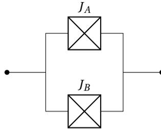
Figure 2.4: SQUID loop circuit component.
