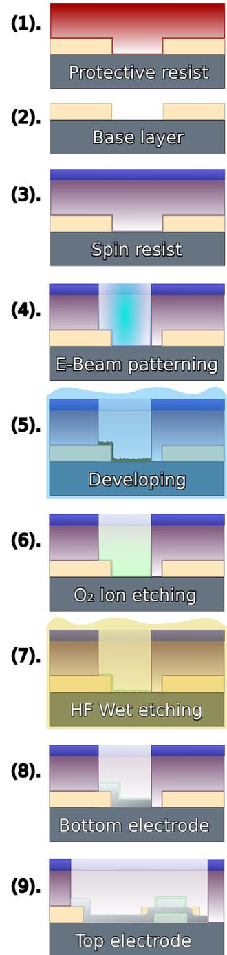
Figure 3.2: Fabrication process flow for a die with JJs, picture greatly inspired and adapted from [29, p. 21].
