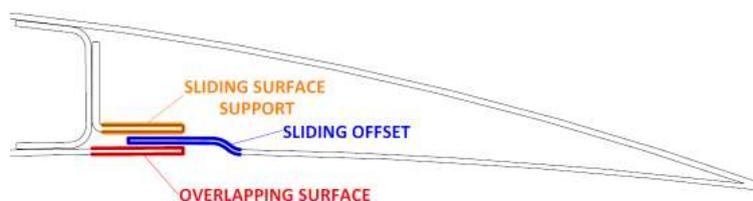
Figure 2.2: Critical features to be included in the design to achieve TRIC morphing
