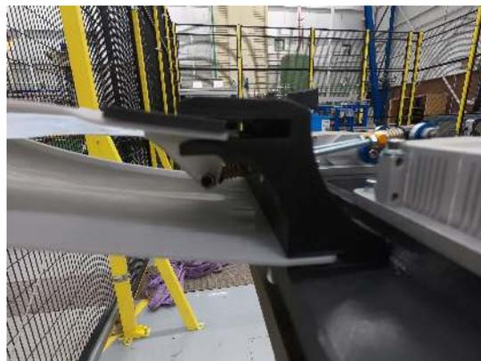
Figure 7.11: Pivoting effect witnessed under actuation, shown in the elastomer test setup during a camber morphing configuration
