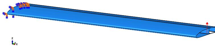
Figure 3.39: Wingbox and leading edge analysis
