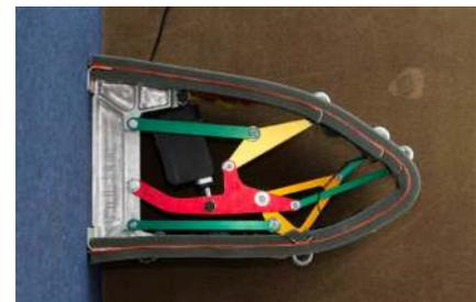
Figure 1.2: Droop nose morphing demonstrator used in experimental evaluation by Sodja et al. [46]
