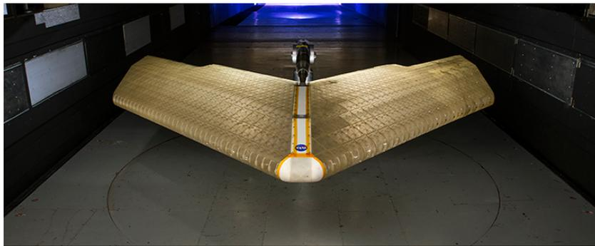
(a) MADCAT morphing wing which was built from assembly of many small building blocks [23]
