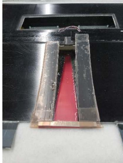
Figure 5.17: Application of the silicone on top wing surface through the underside of the wing
