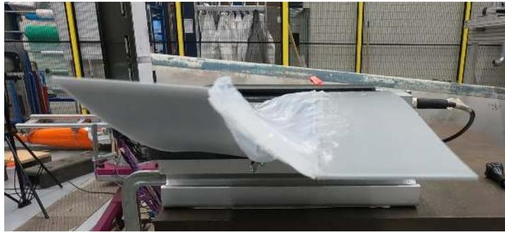
Figure 5.15: Peak anti-symmetric tip deflections captured on the final prototype
