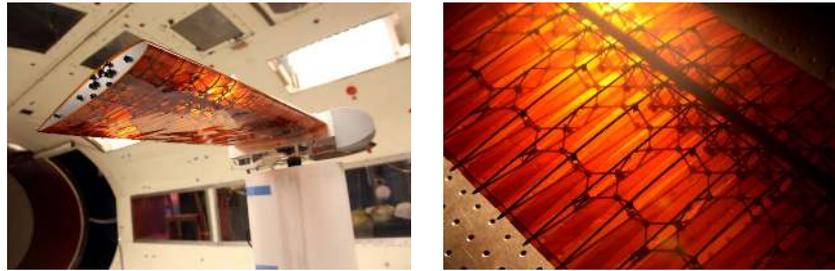
(b) Digital morphing wing concept with a lattice based structure [14]
