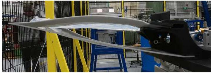
Figure 5.12: Bulging effect seen on the second prototype during anti-symmetric actuation
