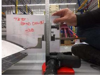
Figure 7.3: Rudimentary test setup to measure trailing edge tip deflections with a Vernier scale height gauge
