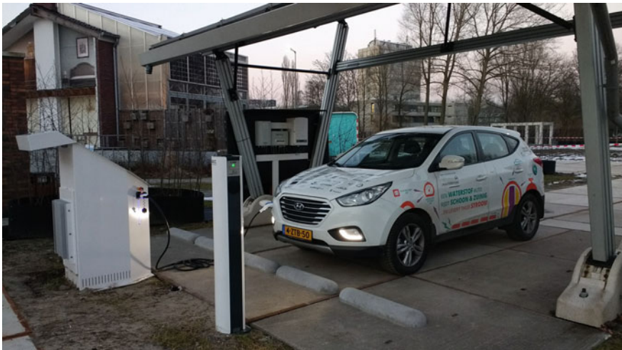
Fig. 8.3 Photo of the modified Hyundai ix35 FCEV connected to the grid through the V2G unit at The Green Village in The Netherlands
