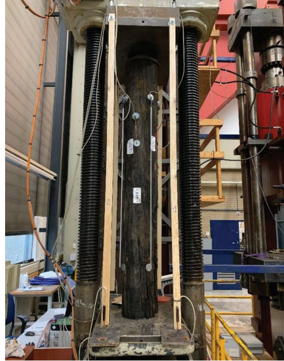
Figure 2: Setup for compression tests.
