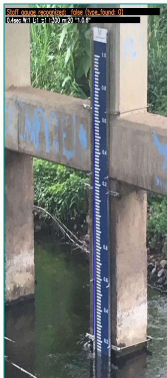
Fig. 4.4: Incorrect sticker alignment (Location 9)
