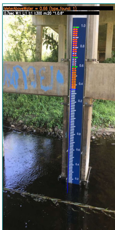
Fig. 5.2: Incorrect sticker alignment
