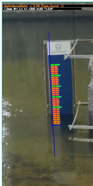
Fig. 4.5: Staff gauge water reflection (Location 6)
