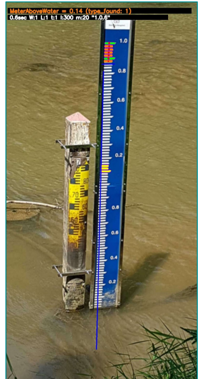
Fig. 4.3: Incorrect sticker alignment (Location 4)
