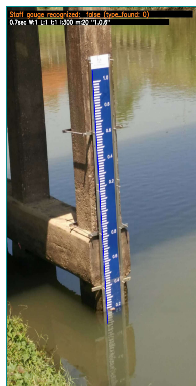
Fig. 5.3: Staff gauge not recognized
