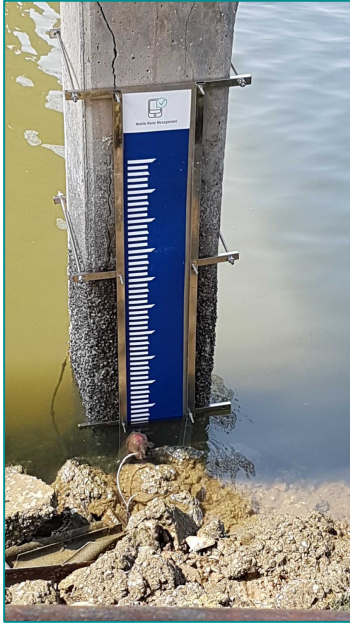
Fig. 3.3: Staff gauge at Location 1
