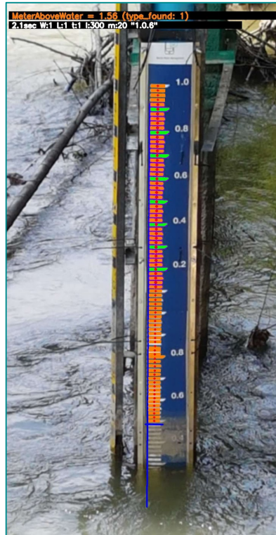
Fig. 4.2: Sedimentation on staff gauge (Location 3)
