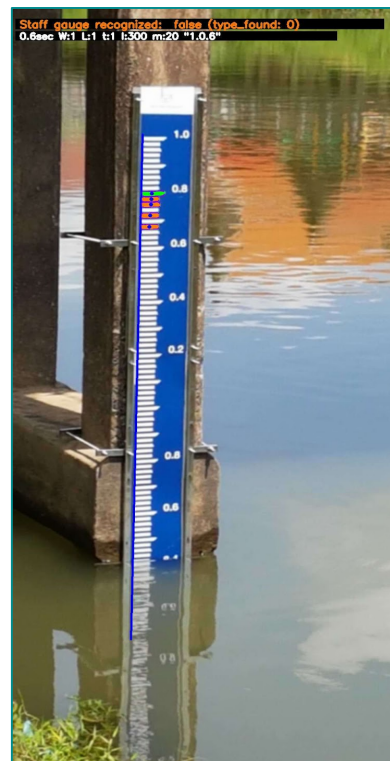
Fig. 4.6: Staff gauge water reflection (Location 2)
