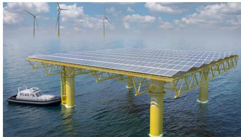
**Figure 4.3:** The Seavolt concept on which the model is based
