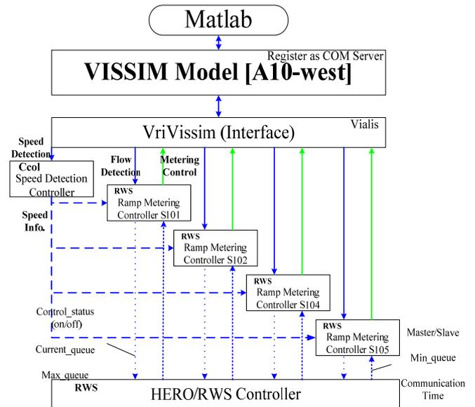
Fig. 2. VISSIM simulation environment (blue lines indicate data streams; green lines indicate control streams).
