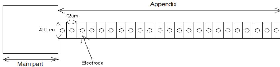
Figure 3.7: Cochlear implant with electrodes and dimensions of the electrodes
