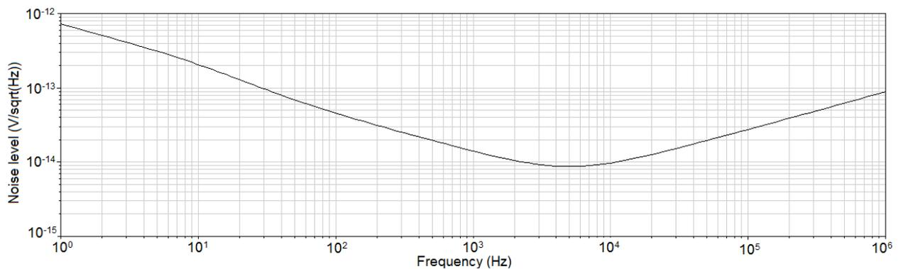
Figure 7.19: Noise simulation of the charge offsetting circuit
