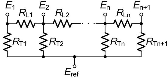
Figure 2.5: Resistor network of cochlear tissue
