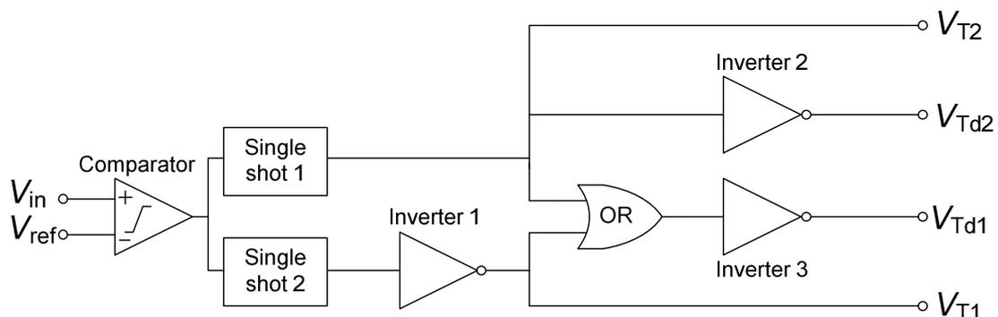
Figure 6.9: Control loop for subtracting charge
