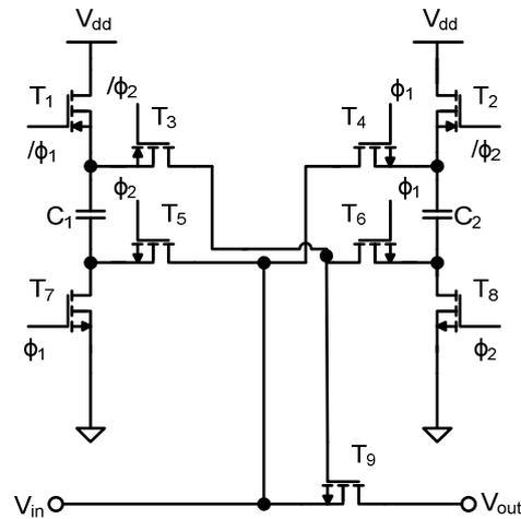
Figure 7.9: Practical clock bootstrapping circuit
