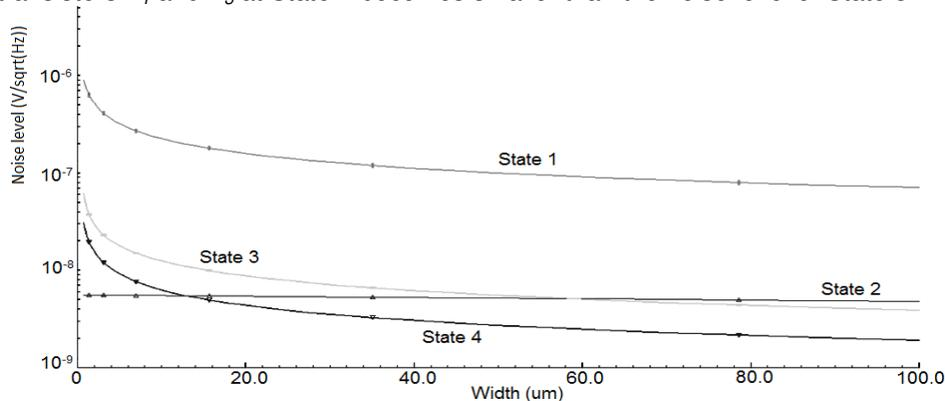
Figure 5.13: Transistor width variation for 4 different states
