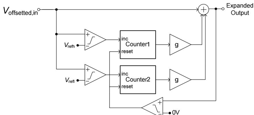
Figure 5.17: Simulink schematic for expanding the offsetted signal
