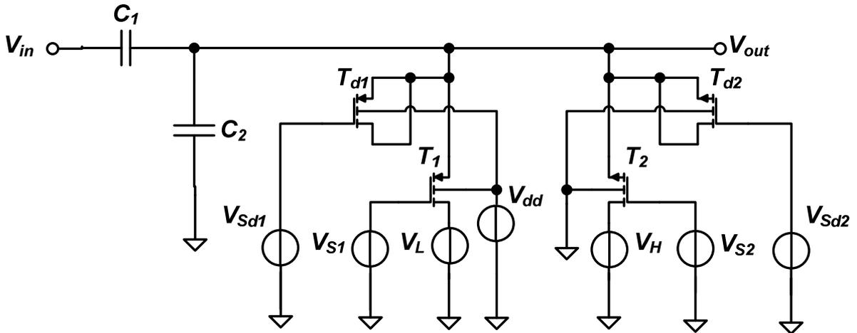
Figure 5.8: Circuit with dummy transistors
