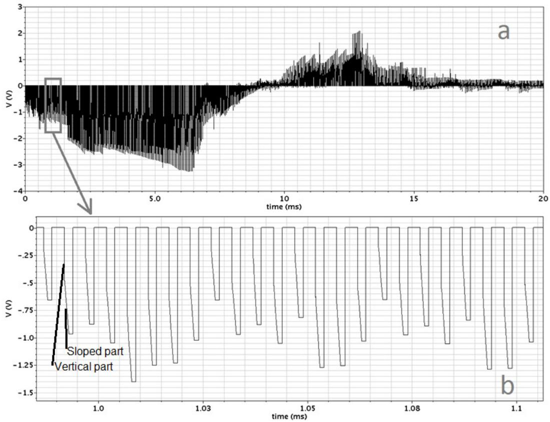
Figure 3.18: Output of amplifier  $G_1$
