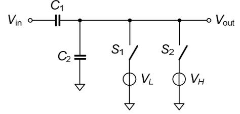
Figure 4. Voltage controlled offsetting circuit
