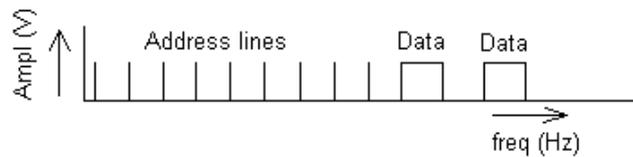
Figure 3.10: Addressing and data at one single wire
