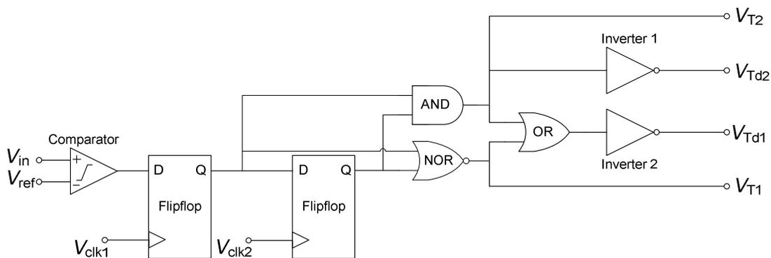
Figure 6.12: Practical charge subtracting circuit
