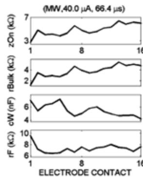
Figure 2.9: Electrode model component values per stimulation site stimulated with pulses with 66.4μs pulse width [17].
