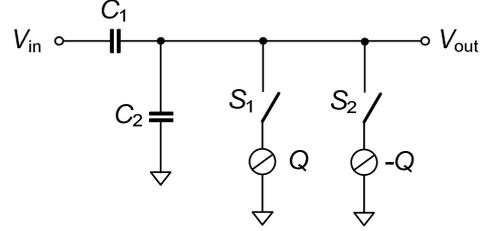
Figure 5. Charge controlled offsetting circuit
