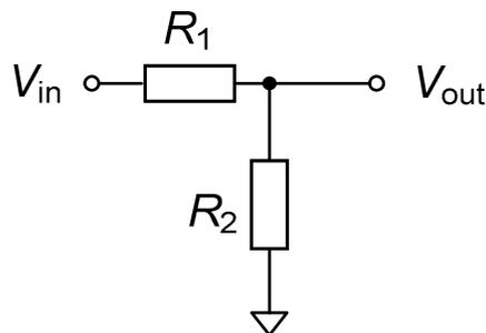
Figure 4.1: Resistive dividing network
