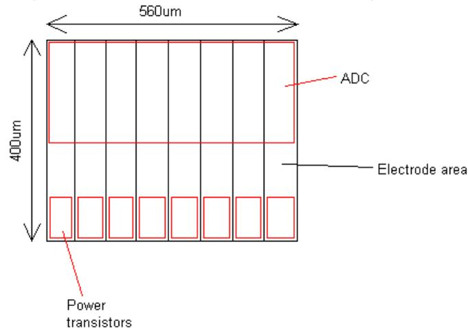
Figure 3.12: Chip area arrangement of the ADC and power transistors spread over 8 electrodes
