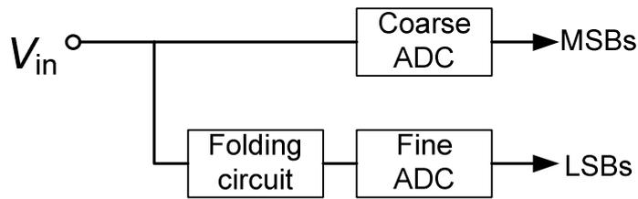
Figure 4.6: System block schematic of a folding ADC
