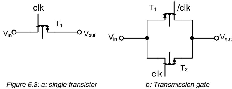
Figure 6.3: a: single transistor
