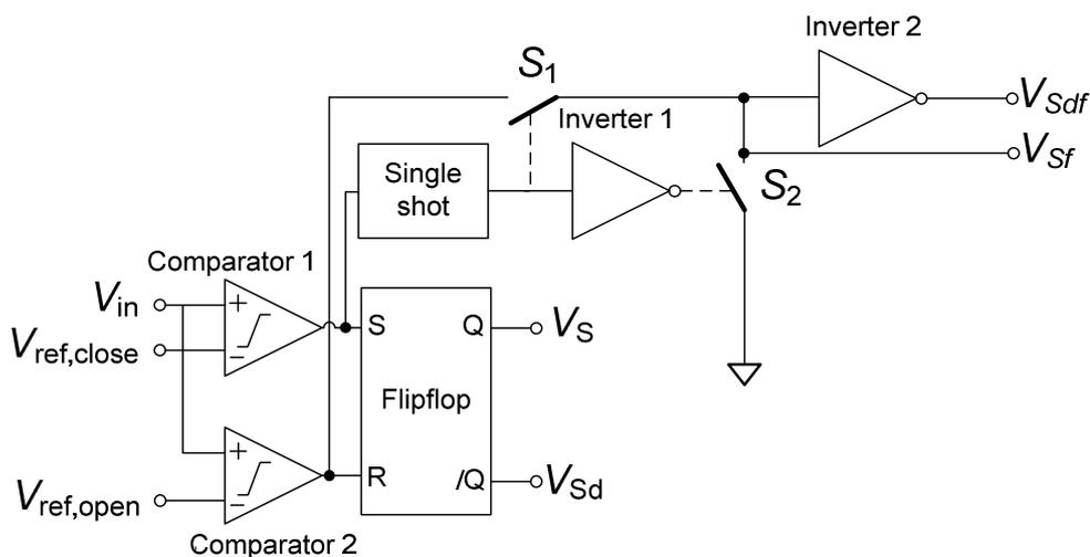
Figure 5.12: Control loop with course and fine offsetting ability
