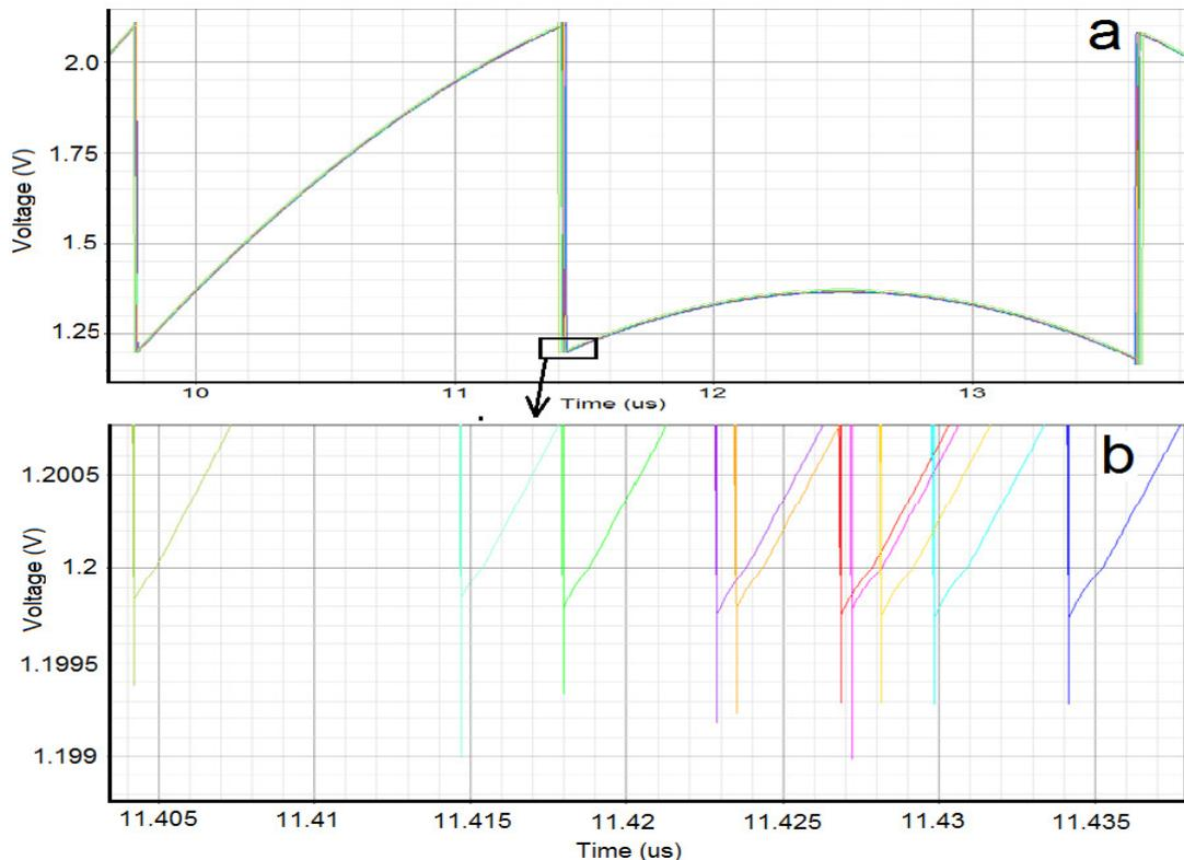
Figure 5.20: Temperature simulation of the offsetting circuit
