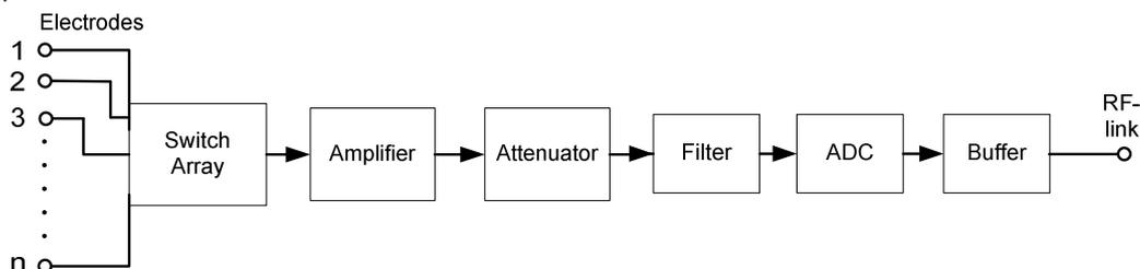
Figure 3.2: System block diagram of the front-end of the implant
