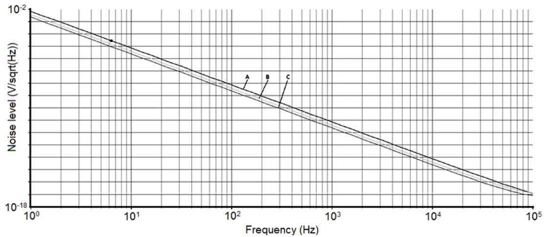
Figure 6.14: Noise analysis of the implemented circuit with implemented control loop
