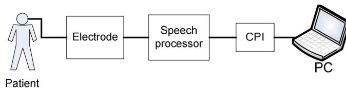
Figure 3.1: Block-system diagram of the front-end for advanced bionics implants [37]
