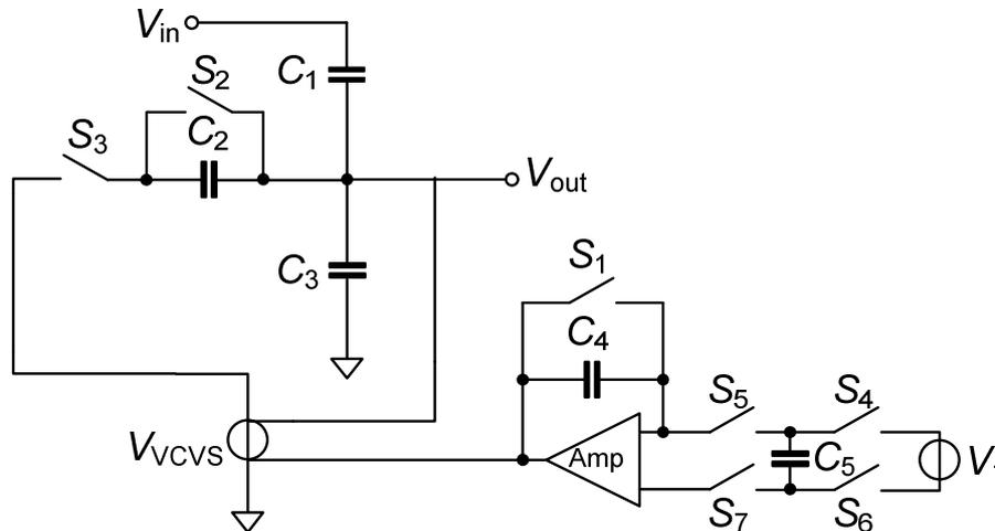
Figure 7.4: Charge injection circuit with a charge amplifier having a fixed reference
