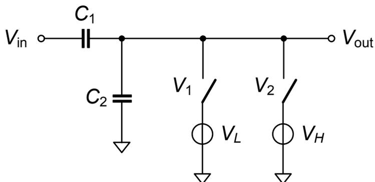
Figure 4.12: Schematic of the blanking capacitor concept
