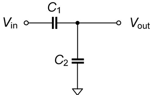
Figure 4.11: Capacitive divider
