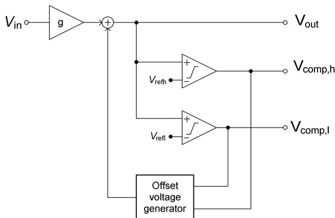
Figure 4.9: system-block diagram of the input attenuator
