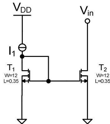
Figure 7.14: Practical current mirror for biasing
