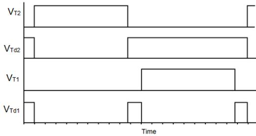
Figure 6.10: Control signals applied to NMOS transistors
