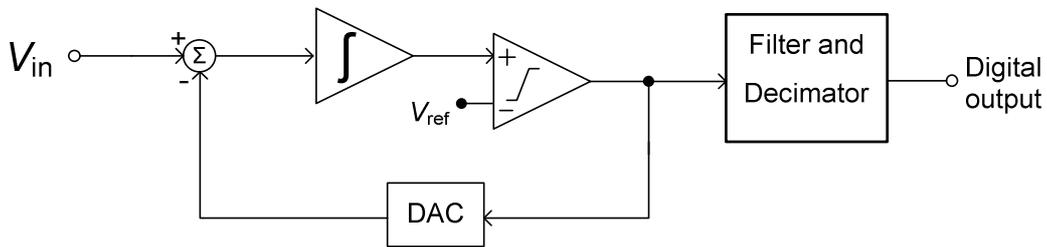
Figure 4.8: System block diagram of a  $\Sigma\Delta$  converter
