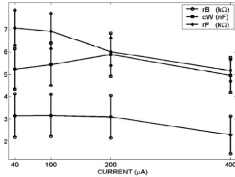
Figure 2.7: component values vs. stimulation current [17].
