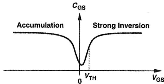
Figure 5.16: Parasitic capacitance versus voltage of a transistor [29]
