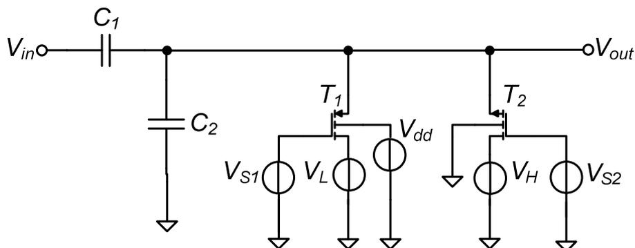
Figure 5.4: The blanked capacitor circuit with non-ideal components
