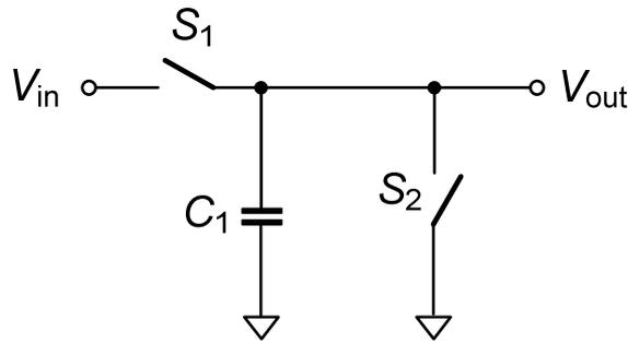
Figure 4.2: Conventional switched capacitor circuit
