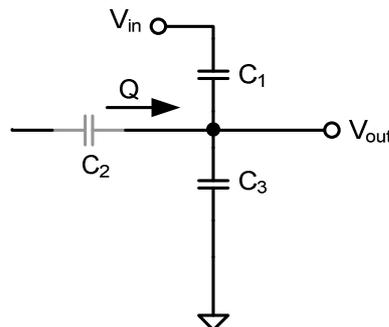
Figure 7.1: concept of charge injection in the capacitive divider
