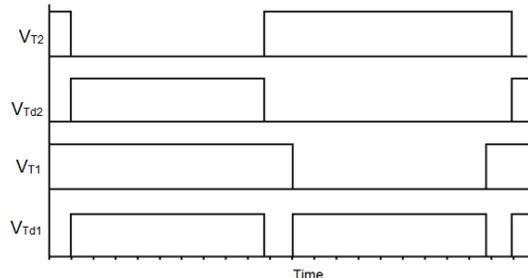
Figure 6.11: Control signals applied to NMOS transistors
