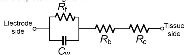
Figure 2.4: Electrical representation of the tissue-electrode interface in the cochlea
