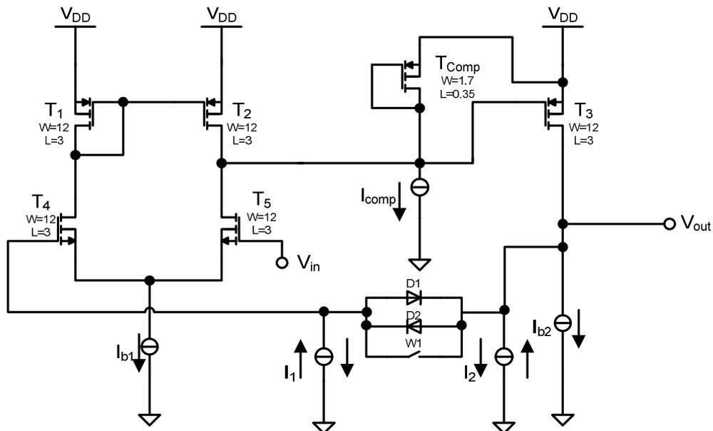
Figure 7.13: Amplifier with practical implementation of frequency compensation
