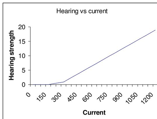
Figure 3.5: Hearing strength versus current
