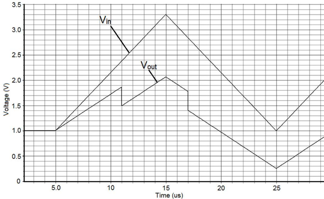
Figure 7.6: Transient simulation of double charge injection circuit with fixed reference amplifier
