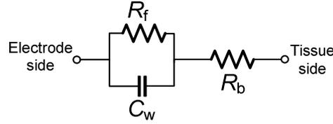
Figure 2.3: Model for the electrode-tissue interface
