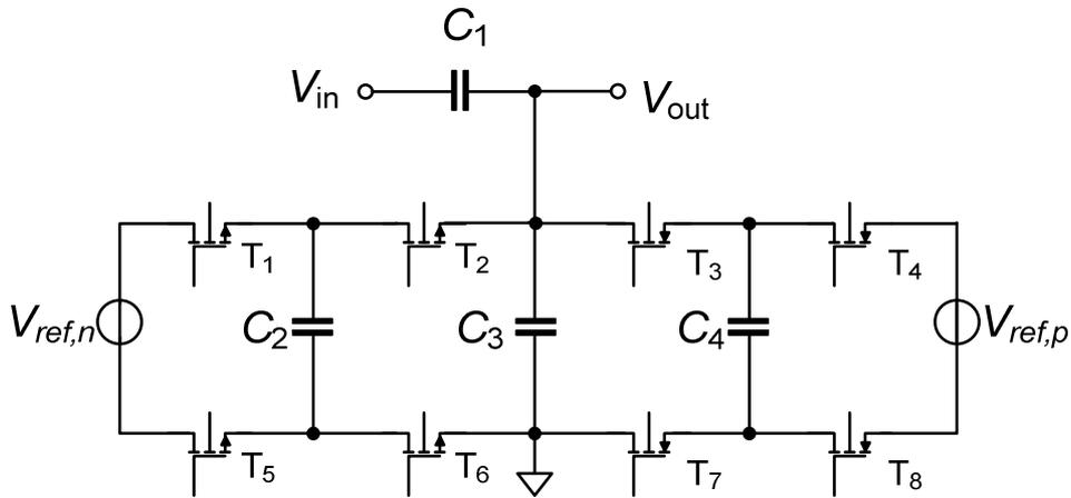
Figure 6.4: Practical circuit for charge offsetting
