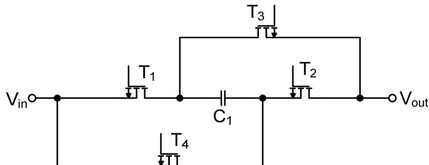
Figure 7.7: Practical implementation of capacitor reversing switches
