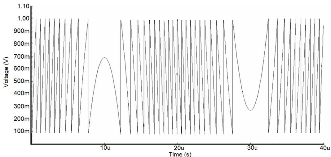
Figure 5.3: Output of the switched capacitor attenuator.
