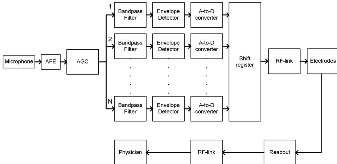
Figure 1.10: Overall architecture of an analog cochlear implant.
