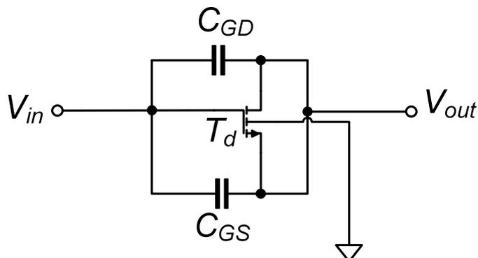
Figure 5.9: dummy transistor with parasitic capacitance
