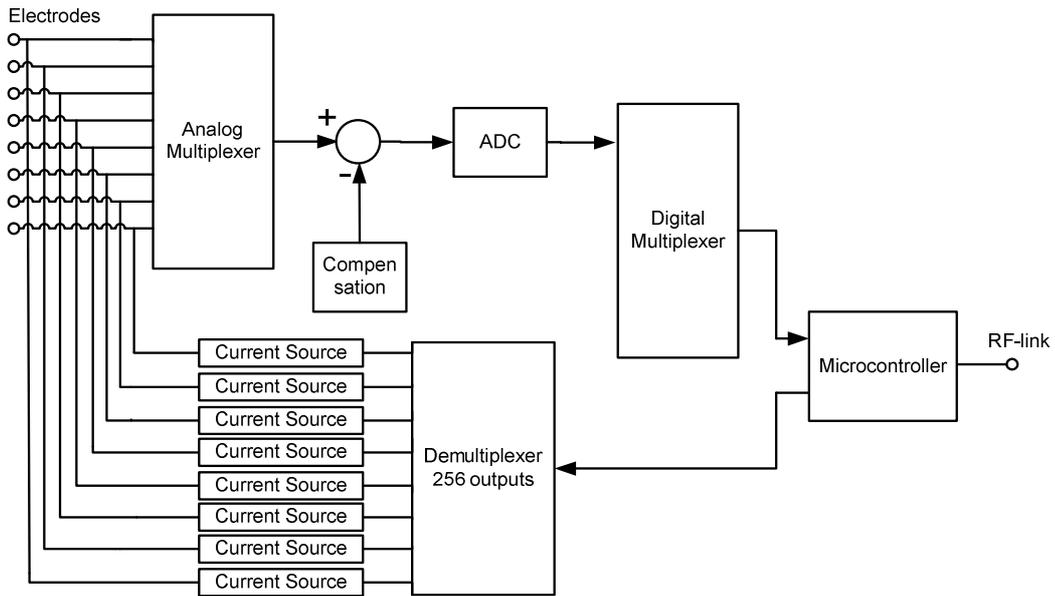
Figure 3.13: High level system-block diagram of the cochlear implant readout and stimulation circuit
