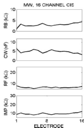
Figure 2.8: Channel number vs. component value at 1kHz [17].
