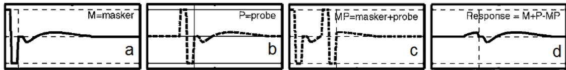
To suppress electrical noise, EMI and action potentials originating from different parts of the human body, many averaging cycles are performed. In practice, up to 512 readout cycles are performed and averaged.
