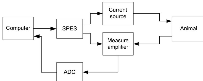
Figure 3.3: System block diagram of the setup used for animal testing with the measure amplifier.
