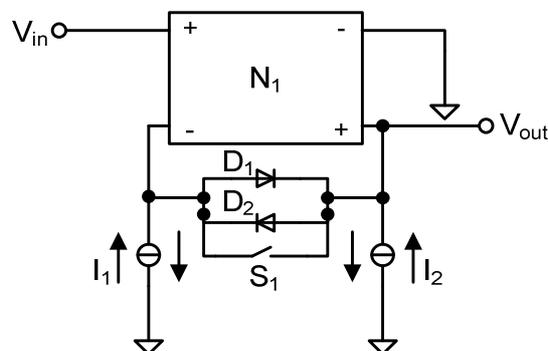
Figure 7.10: Three state amplifier with diodes in feedback loop
