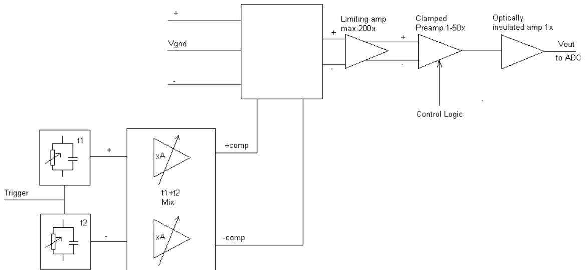
Figure 3.4: Block-system diagram of the amplifier developed at the LUMC used for cancelling stimulus artifact during measurements [10]
