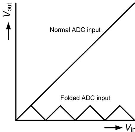
Figure 4.7: ADC input voltages with and without folding
