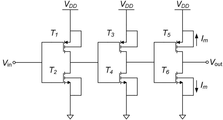
Figure 3.16: Inverter schematic with 3 inverters
