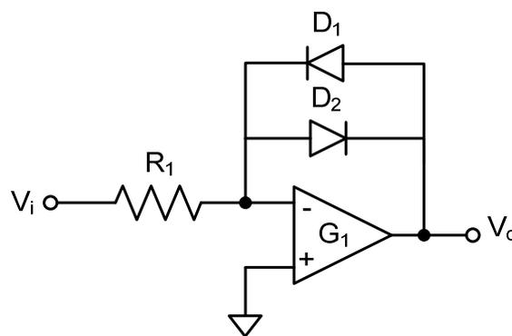
Figure 3.8: Principle of logarithmic amplifier
