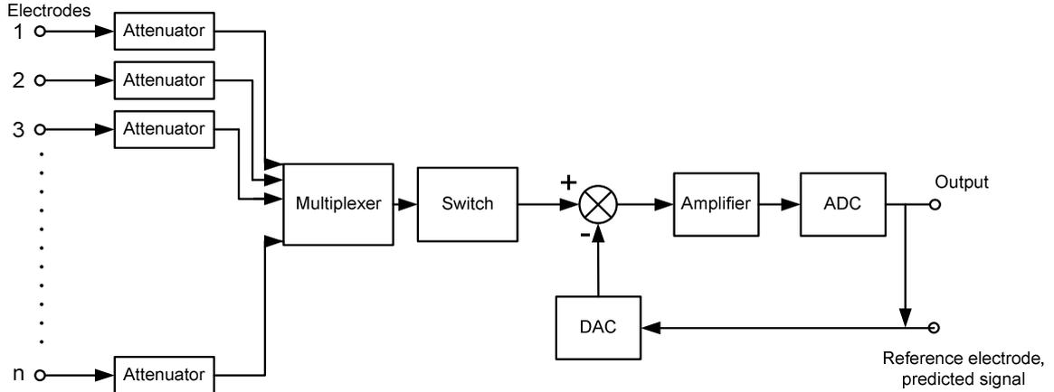
Figure 3.15: Modified system-block diagram of the readout circuit of the cochlear implant
