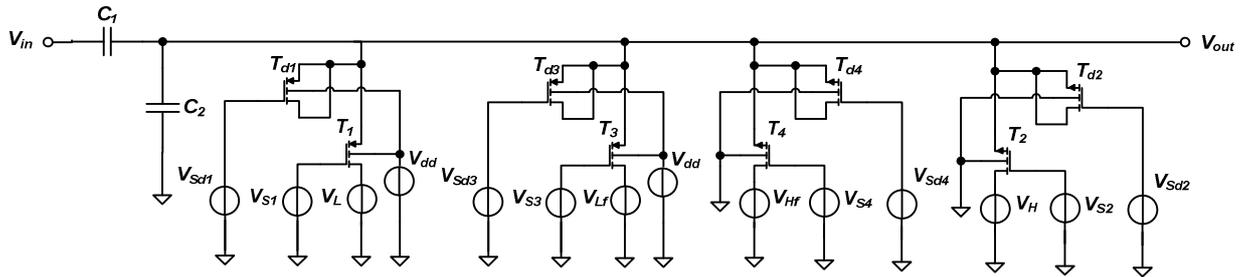
Figure 5.11: Switching circuit with coarse and fine offsetting
