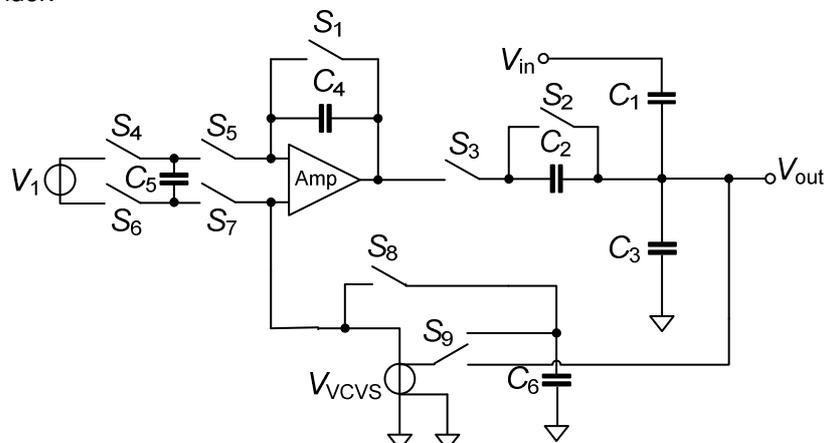
Figure 7.3: Modified floating charge amplifier concept
