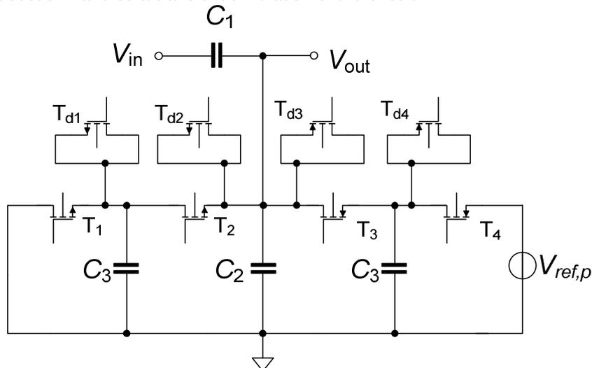
Figure 6.5: Modified practical circuit for charge offsetting
