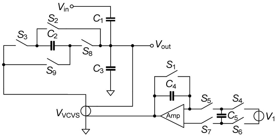
Figure 7.5: Double charge injection circuit with a fixed reference charge amplifier
