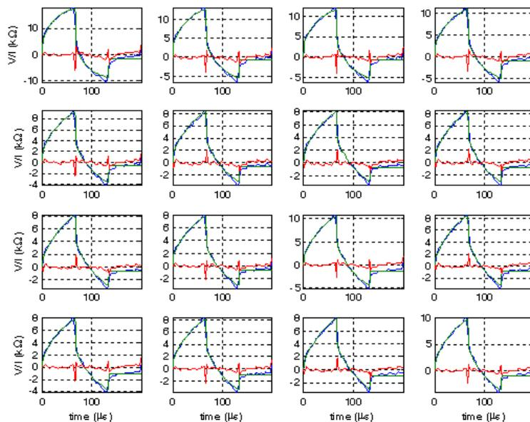
Figure 2.11: Calculated and measured impedance due to stimulus of electrode and the difference between those two [18].
