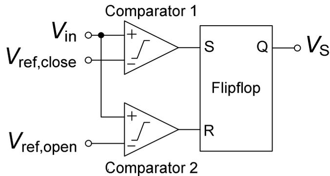
Figure 5.6: Modified control circuit
