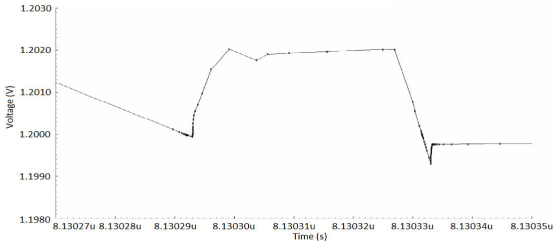
Figure 5.10: Charge injection cancellation at the end of the blanking
