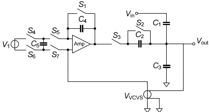
Figure 7.2: Concept of a floating charge amplifier
