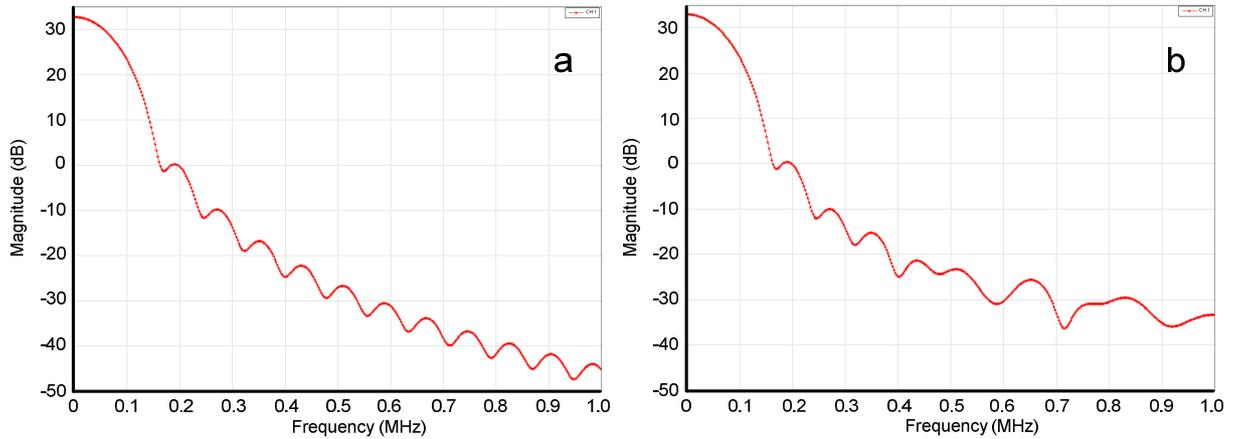
Figure 7.26: Fourier analysis output of a sine wave and of the circuit output
