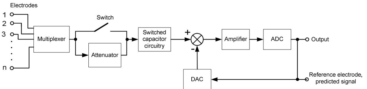
Figure 3.14: Detailed system-block diagram of the readout circuit of the cochlear implant
