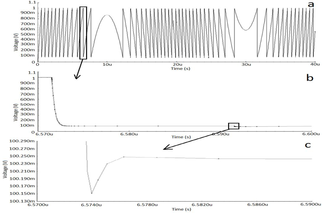
Figure 5.5: Transient output practical switched capacitor circuit
