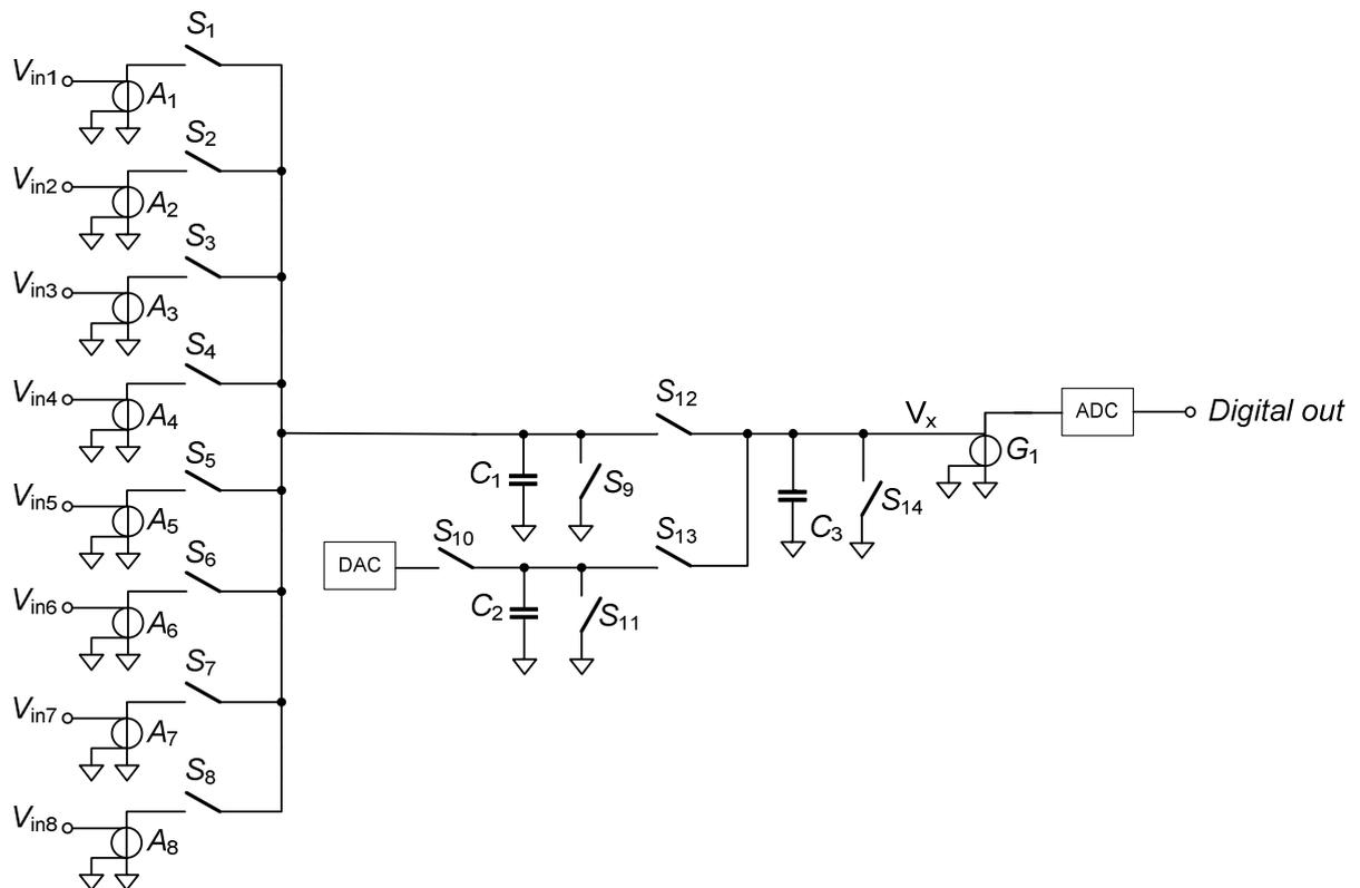
Figure 3.17: High level cadence schematic of the proposed system
