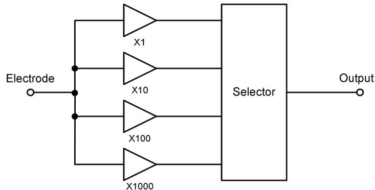
Figure 3.9: Principle schematic of parallel amplifiers
