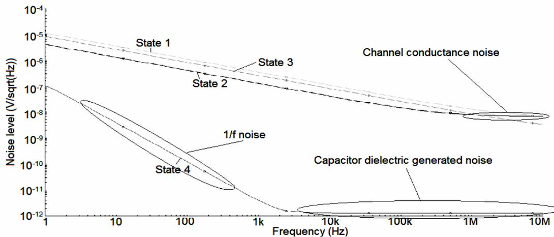
Figure 5.15: Noise simulation of the complete circuit
