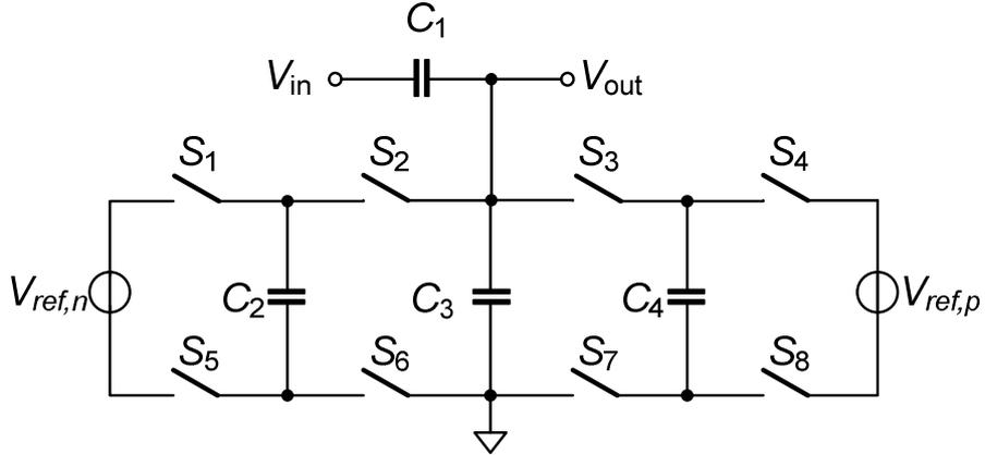
Figure 6.2: Ideal circuit for charge subtraction
