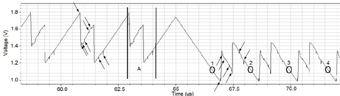
Figure 7.18: Transient simulation of the charge offsetting circuit
