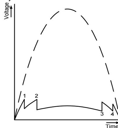
Figure 4.5: Output voltage of the multiplicative companding circuit
