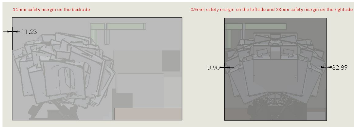
Figure 5-2: Modification of cabin front corner to avoid potential collision with side walls
