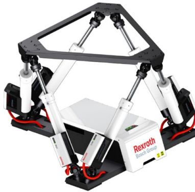
Figure 1-2: System overview of the installed hexapod motion simulator (neutral pose) at MPI[2]
