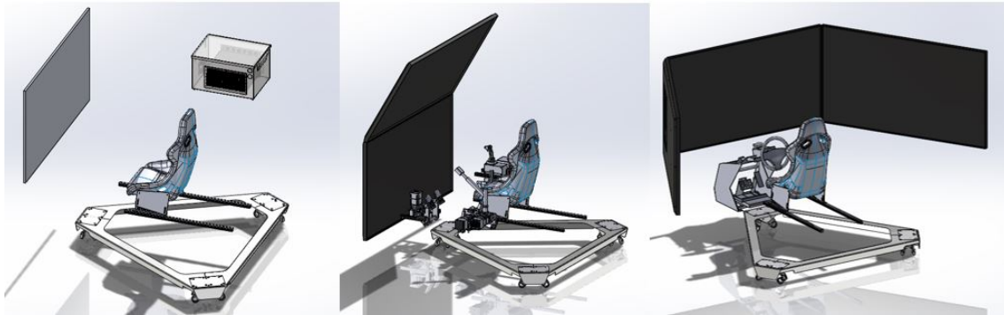
Figure 1-1: Setup required for various experiments: psychophysics (left), helicopter simulation (middle) and car simulation (right)
