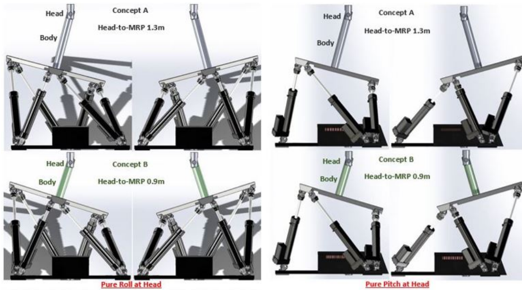
Figure 3-4: Models to check the maximum pure roll and pitch excursion at head with different head-to-MRP distances of 1.3m and 0.9m
