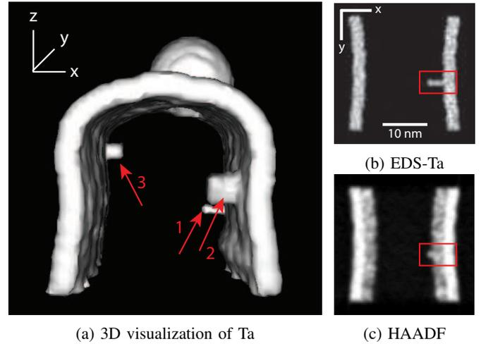
Fig. 5: (a) Volume rendering of the noiseless Ta (tantalum) reconstruction for the simulated finFET dataset; SIRT with 100 iterations using 90 elemental maps between  $[0^\circ, 180^\circ)$ . Three arrows point to the Ta penetration caused by the pinhole defects in the inner  $\text{HfO}_2$  layer. (b) and (c) are the Ta and HAADF reconstruction  $xy$ -slices at  $z = 37$ , corresponding to the first arrow in (a). Red rectangles indicate the defect.
