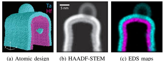
Fig. 2: (a) Atomic design of a defective finFET structure. Tantalum (Ta, cyan) layer and hafnium (Hf, magenta) in  $\text{HfO}_2$  layer are shown for clarity. (b) HAADF-STEM projection and (c) superposed EDS maps at  $2^\circ$ . Since the intensity of HAADF-STEM scales with the atomic number  $Z$ , only Ta ( $Z_{\text{Ta}} = 73$ ) and Hf ( $Z_{\text{Hf}} = 72$ ) are visible but O ( $Z_{\text{O}} = 8$ ) is not. Details in Section IV-A.
