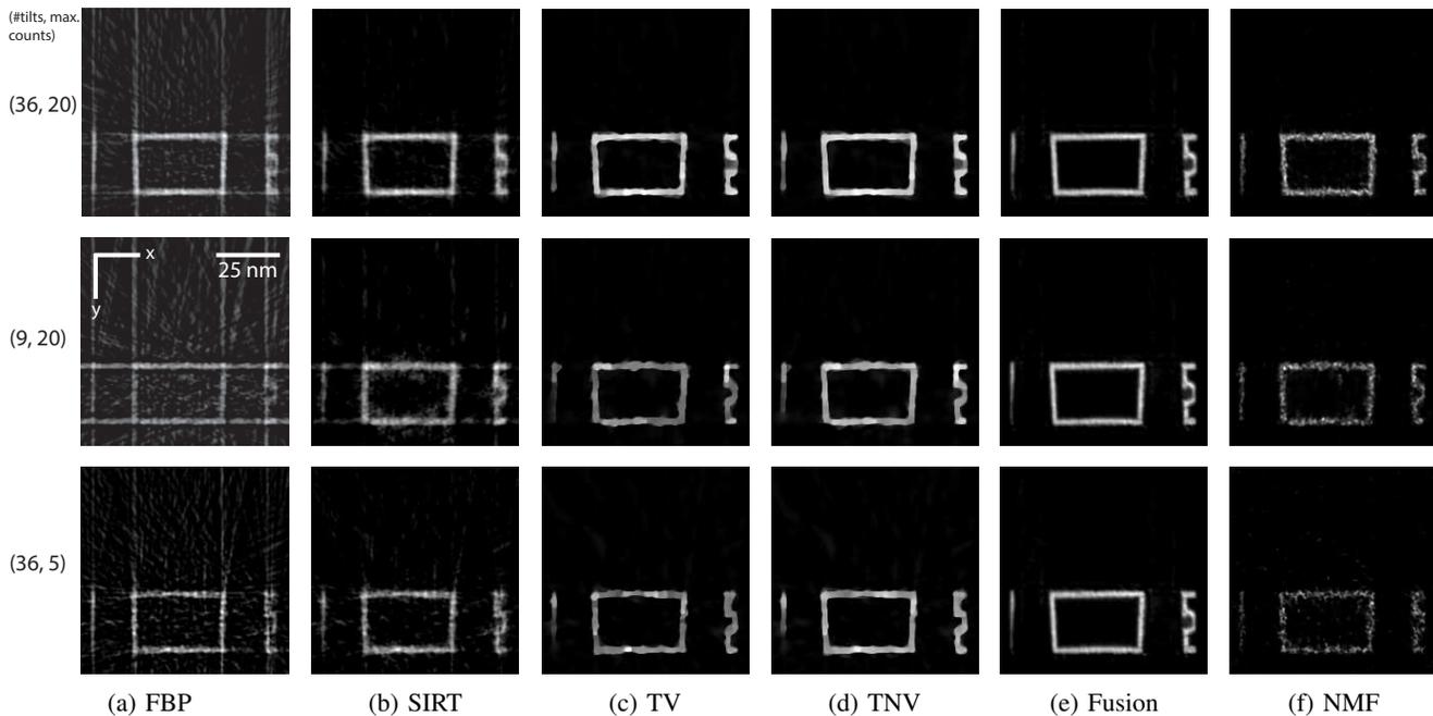
Fig. 8: Ta  $xy$ -slices of (a) FBP, (b) SIRT, (c) TV, (d) TNV, (e) fusion and (f) NMF denoising for the simulated PMOS at  $z = 94$  (the height of the arrow in Fig. 7(a)). The top row is the “normal” case where the number of EDS projections and the maximal X-ray counts per pixel are 36 and 20. Middle and bottom rows are the limited-tilt case (with 9 projections) and low-count case (max. 5 X-ray counts), respectively.
