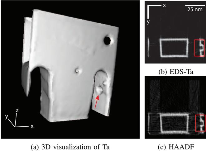
Fig. 7: (a) Volume rendering of the noiseless Ta reconstruction for the simulated PMOS dataset; SIRT with 100 iterations using 72 elemental maps between  $[0^\circ, 180^\circ]$ . (b) and (c) are the Ta and HAADF reconstruction  $xy$ -slices at  $z = 94$ , in which red rectangles encompass a fine structure indicated by the arrow in (a).
