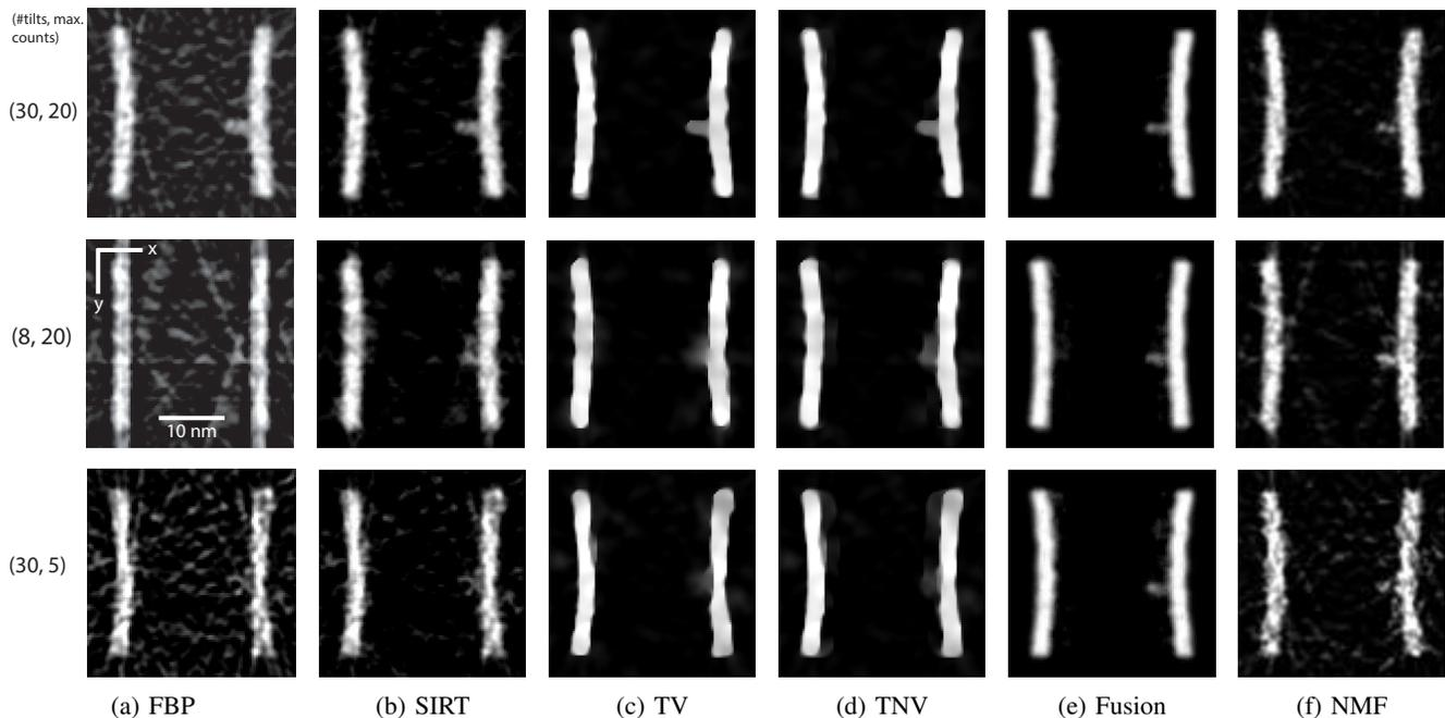
Fig. 6: Ta  $xy$ -slices of (a) FBP, (b) SIRT, (c) TV, (d) TNV, (e) fusion and (f) NMF denoising for the simulated finFET at  $z = 37$  (the height of the first defect in Fig. 5(a)). The top row is the “normal” case where the number of EDS projections and the maximal X-ray counts per pixel are 30 and 20. Middle and bottom rows are the limited-tilt case (with 8 projections) and low-count case (max. 5 X-ray counts). For better visualization, we perform percentile contrast stretching from 0 to 99%.
