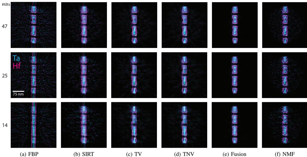
Fig. 10: Superposed  $xy$ -slices of Ta (cyan) and Hf (magenta) reconstructions computed by (a) FBP, (b) SIRT, (c) TV, (d) TNV, (e) fusion and (f) NMF denoising for the experimental dataset using 47 (top), 25 (middle) and 14 (bottom) EDS projections.
