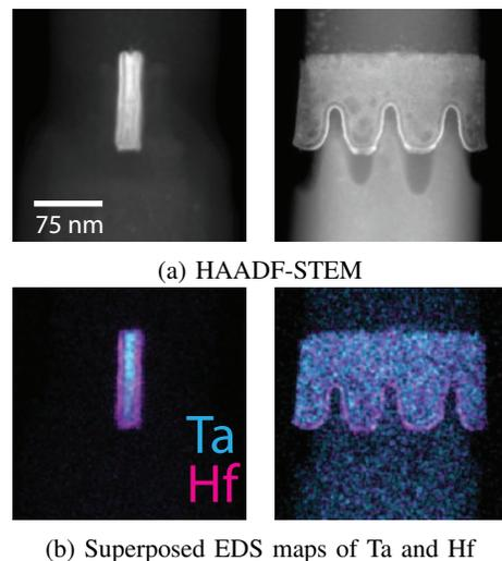
Fig. 4: Experimental (a) HAADF-STEM projections and (b) EDS maps of a pillar-shaped semiconductor device at  $0^\circ$  (left) and  $90^\circ$  (right). Titanium with an atomic number of  $Z_{\text{Ti}} = 22$  is surrounded by tantalum (cyan,  $Z_{\text{Ta}} = 73$ ) and hafnium (magenta,  $Z_{\text{Hf}} = 72$ ). Details in Section IV-A.
