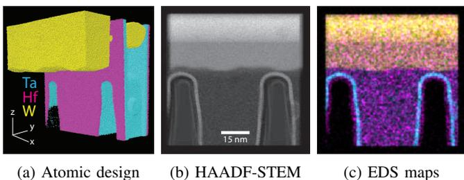
Fig. 3: (a) Atomic design of a PMOS model where tantalum (Ta, cyan), hafnium (Hf, magenta) and tungsten (W, yellow) are shown. (b) HAADF-STEM projection and (c) superposed EDS maps at  $2.5^\circ$ . Ta ( $Z_{\text{Ta}} = 73$ ), Hf ( $Z_{\text{Hf}} = 72$ ) and W ( $Z_{\text{W}} = 74$ ) are clearly visible in the HAADF-STEM image. Details in Section IV-A.
