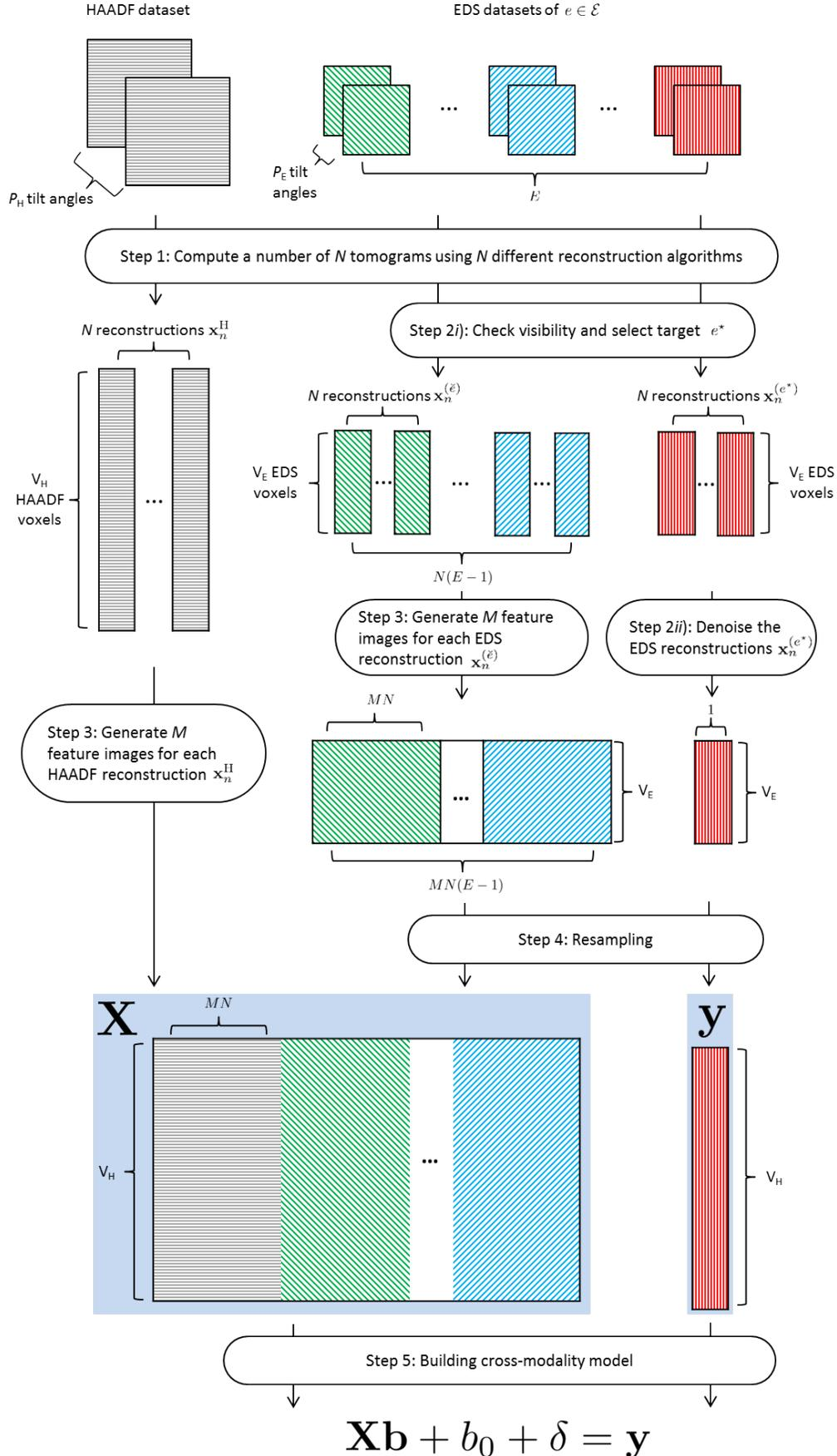
Fig. 1: The first five steps of fusion algorithm. Assume the sample of interest is composed of a set of chemical elements  $\mathcal{E}$ . Denote the target element chosen for fusion as  $e^*$ , and the rest  $\tilde{e} : e \in \mathcal{E} \setminus e^*$ . H symbolizes HAADF and E EDS. Details in Section III.
