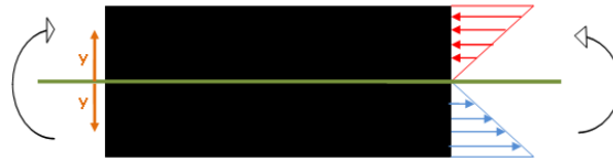
Figure 3.20: Determination of maximum bending inside a root
