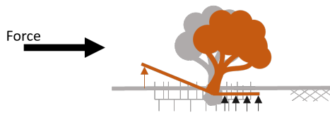
Figure 3.6: Windward uplift of a mangrove tree
