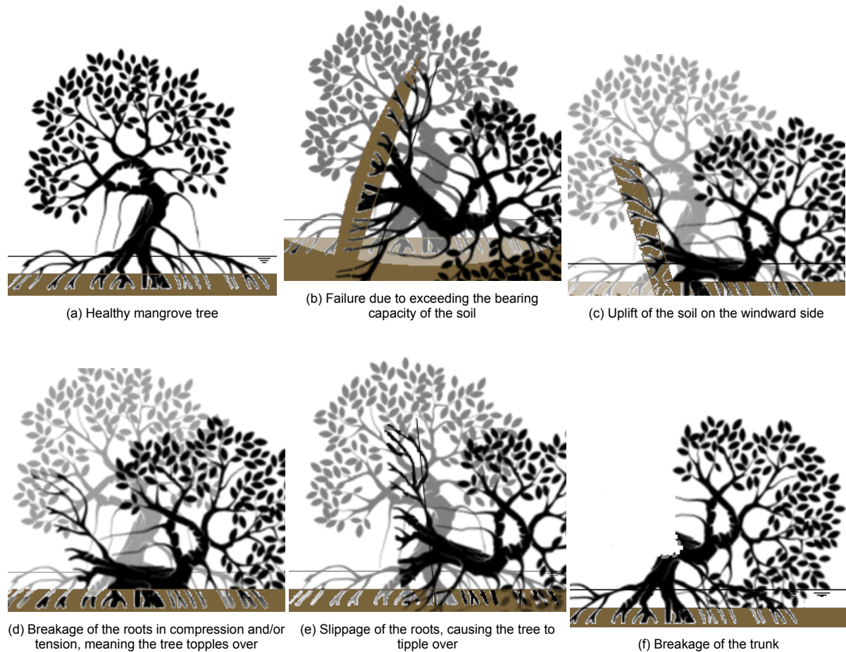
Figure 3.2: Failure mechanisms of the mangrove trees which will be analysed in this report
