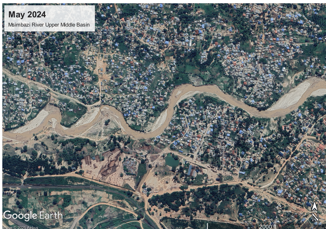
Figure 3.7: Observed river morphology on May 3, 2024. The river appears to have widened further, as shown by houses now located directly along the riverbanks. It should also be noted that the number of buildings has increased considerably between Figures 3.2 and 3.7.
