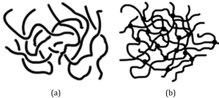
Figure 2.3 Schematic representation of the molecules of (a) the uncrosslinked polymer and (b) the crosslinked polymer (links are pictured as knots), adapted from (Mark et al. 2013).
