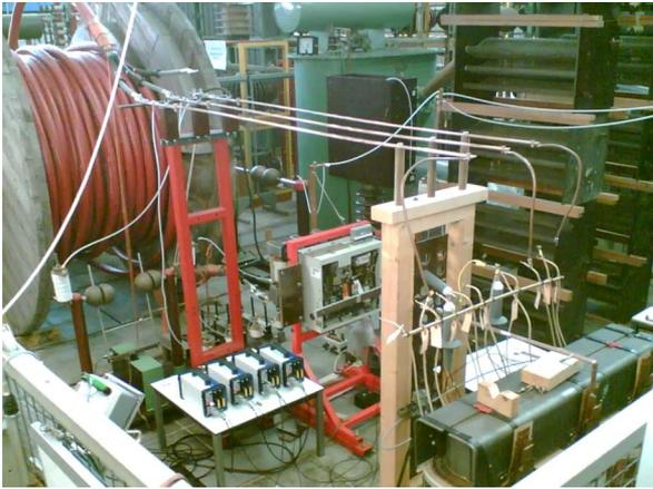
Fig. 7. Transformer switching test circuit.
