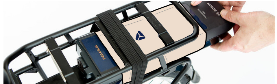
Figure 118: The rear rack battery model [52]
