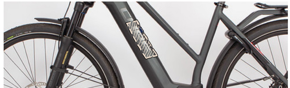
Figure 117: The fixed in-frame battery model [52]
