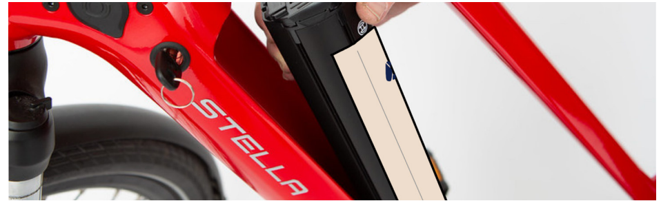
Figure 116: The hidden in-frame tubing battery model [52]
