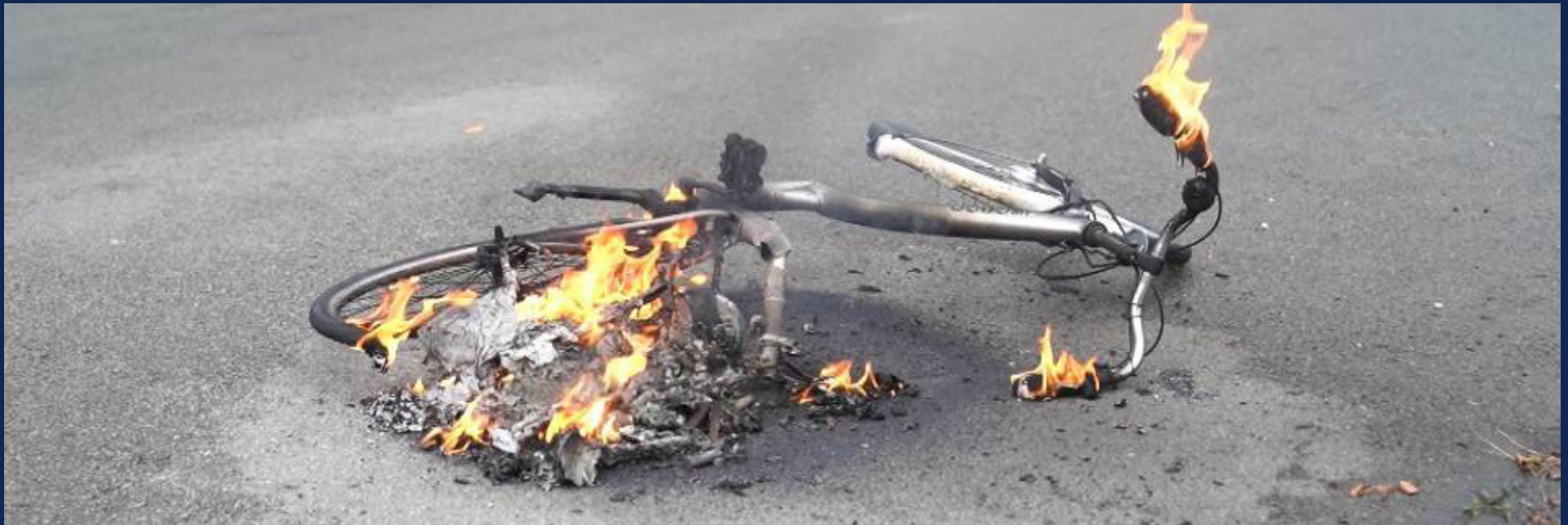
Figure 30: Thermal runaway in action [106]
