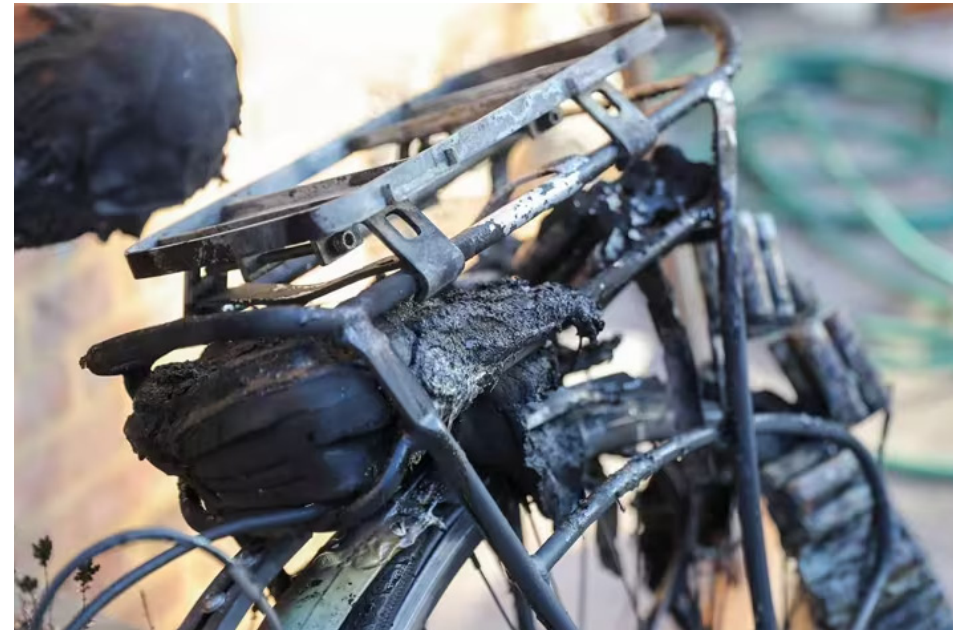
Figure 7: E-bike battery burnt out [16]
