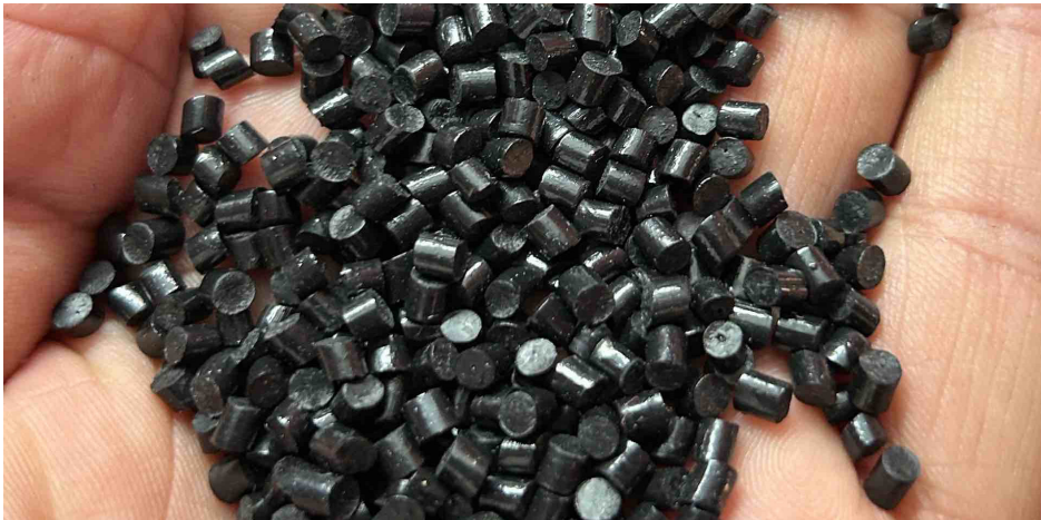
Figure 48: ABS granules before used in the injection molding process to form the e-bike battery shell [121].
