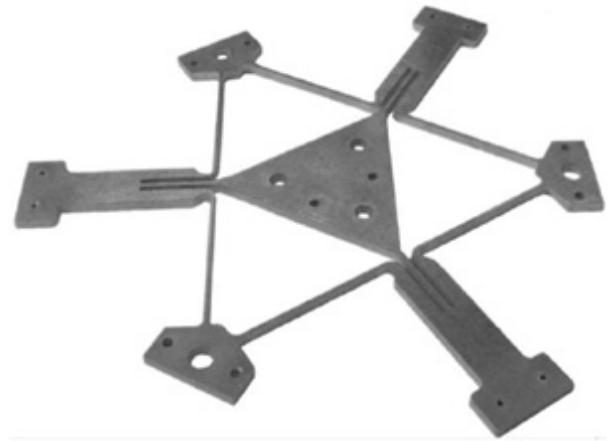
Figure 6. Typically example of a planar compliant stage (Anderson, 2003; Culpepper, 2006; Culpepper and Anderson, 2004). The flexures to perform motion are in the same plane.
