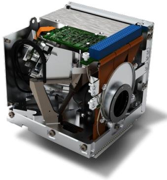
**Figure 2.3:** CUBECAT laser communication terminal from Hyperion Technologies (Engelen, 2020a).
