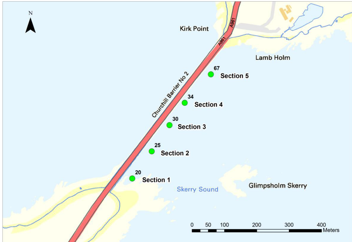
Figure 2.4: Five sections along barrier No. 2, divided by overtopping rate
