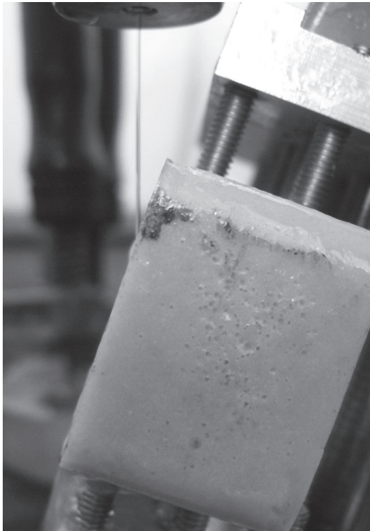
Figure 2. Water jet at 20° applied at specimen C and D.
