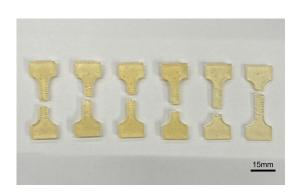
Figure 7.7: Mode 1 failure of the samples
