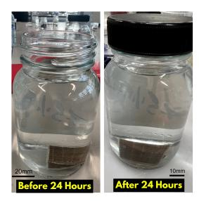
Figure 7.2: Flax/TPU Before and after 24hrs immersion in distilled water
