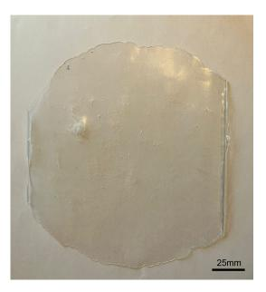
Figure 6.2: Film 2 has many voids in the center of the film
