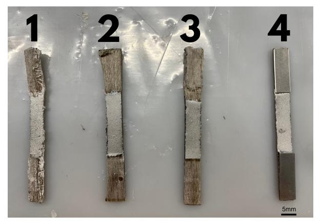
Figure 7.10: Result of 4 Tensile tested samples, sample 1 & 2 using hydraulic clamps, sample 3 with a mechanical clamp and sample 4 using aluminum tabs & mechanical clamps
