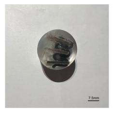
Figure 4.6: Sample prepared for microscopy after grinding and polishing
