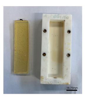
Figure 4.2: TPU pellets after melting and cooling into a block
