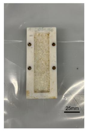
Figure 4.1: TPU pellets placed inside Teflon mould
