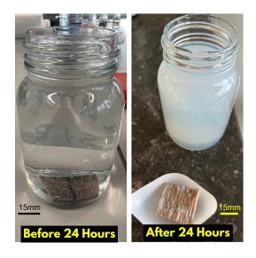
Figure 7.3: Flax/SBPU Before and after 24hrs immersion in distilled water
