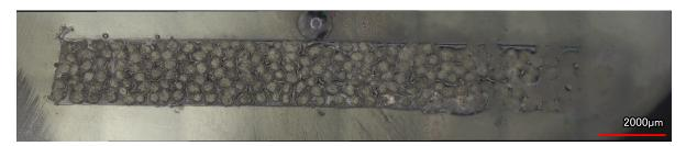
Figure 7.18: Morphology of the Flax/TPU composite at 2x magnification
