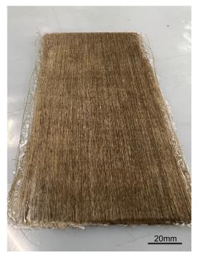
Figure 6.12: Natural fibre composite film stacked after placing under the press
