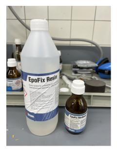
Figure 4.5: EpoFix resin and hardener
