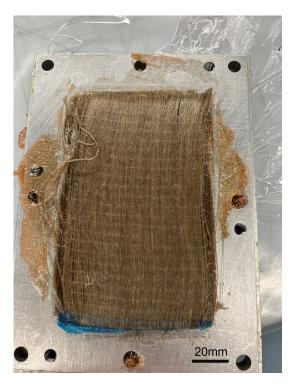
Figure 6.14: Natural fibre composite film stacked after placing under the press
