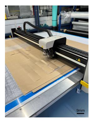
Figure 6.9: Gerber cutting machine cutting out flax fibres in transverse direction
