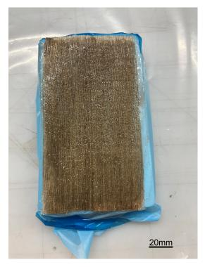
Figure 6.15: Flax SBPU composite after removal from the oven
