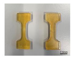
Figure 4.3: TPU dog bone sample ready to be tested
