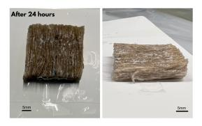
Figure 7.5: Flax/SBPU after 24hrs immersion in distilled water
