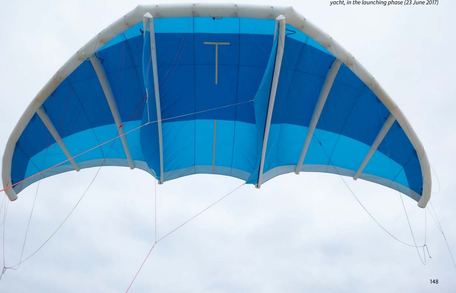
The 50 m 2 kite which is installed on the "Energy Observer" yacht, in the launching phase (23 June 2017)
