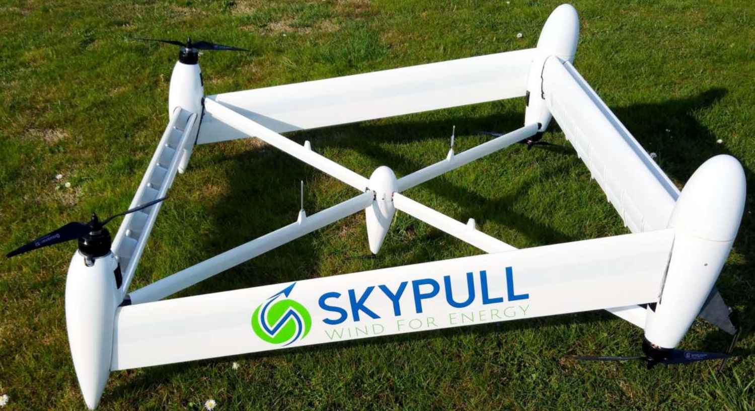
Skypull prototype SPI 125a, 1 kW power system drone (2 March 2016)
