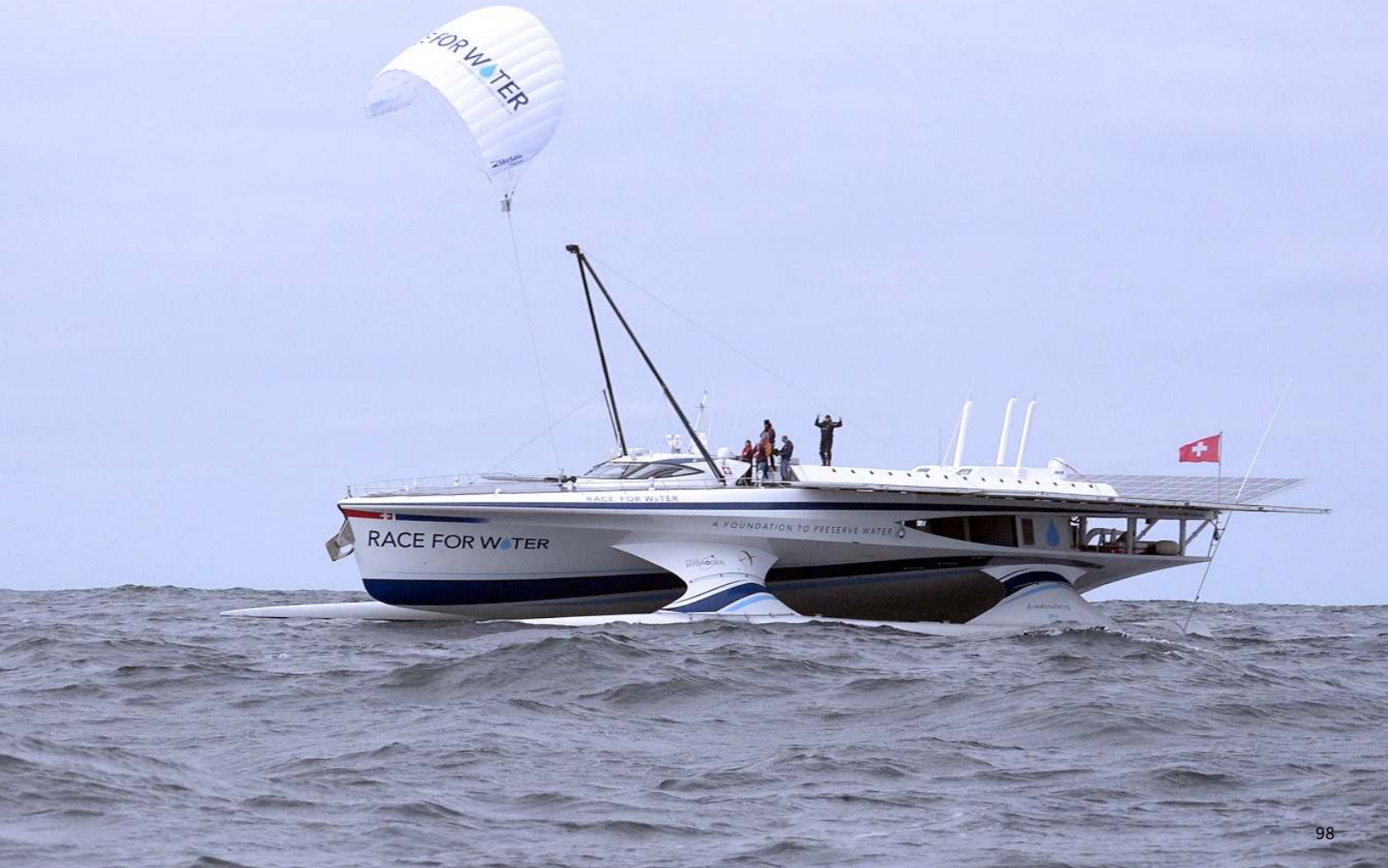
SkySails towing kite being launched from catamaran Race for Water (May 2017)
