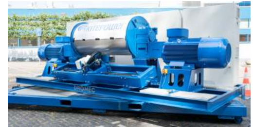
Kitepower "Model A" ground station with 180 kW peak power
