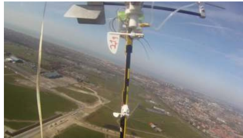
In-flight measurement of apparent wind speed and inflow angles (24 March 2017)
