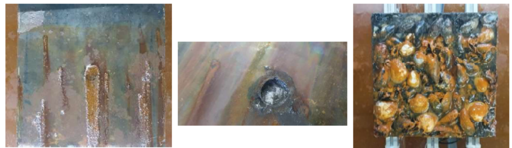
Figure 13. Marine growth covered plate after three weeks of accelerated corrosion.
