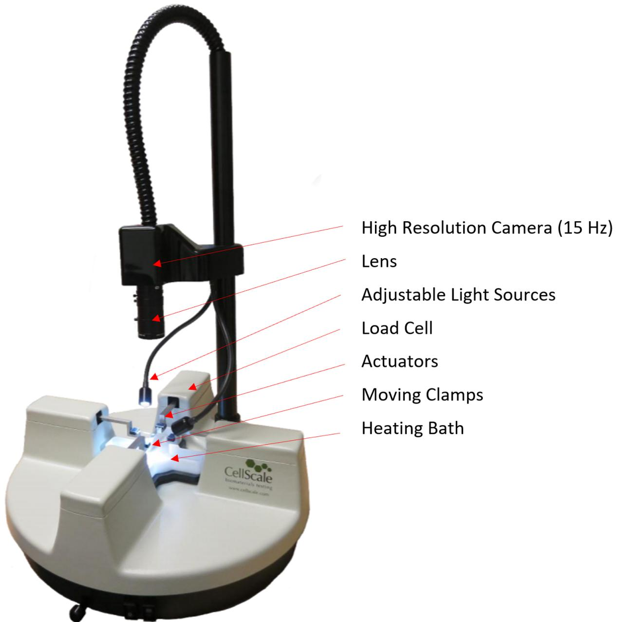
Figure 35: Uniaxial mechanical testing setup with components pointed out [Biomaterial Testing, Waterloo, Canada].
