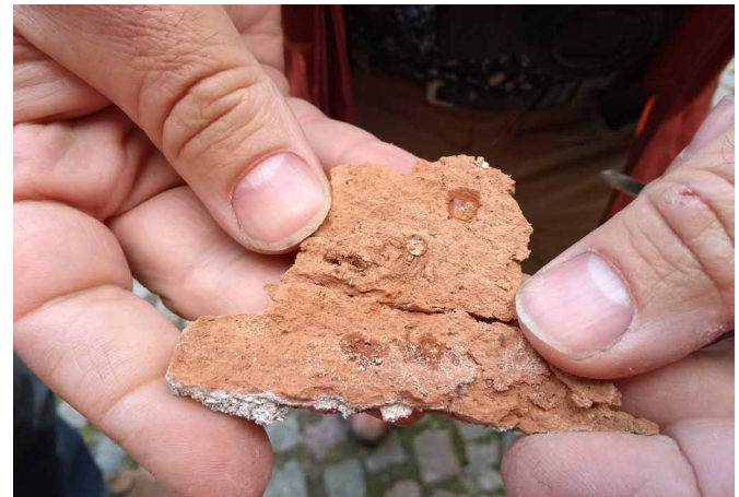
FIGS. 4.14/4.15 Spalling due to salt accumulation beneath the treated layer; the water repellent is still effective several years after the application / Photos: M. van Hunen
