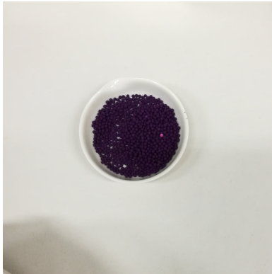
(c) Sample of impregnated Alumina dried prior to calcination
