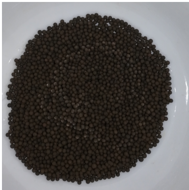
(e) Prepared catalyst after calcination
