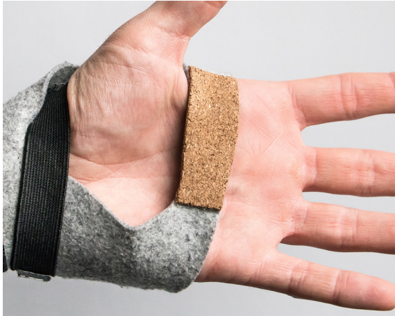
Fig 6.8 | The strip inside the user's hand will tick against the user's hand to ask for feedback
