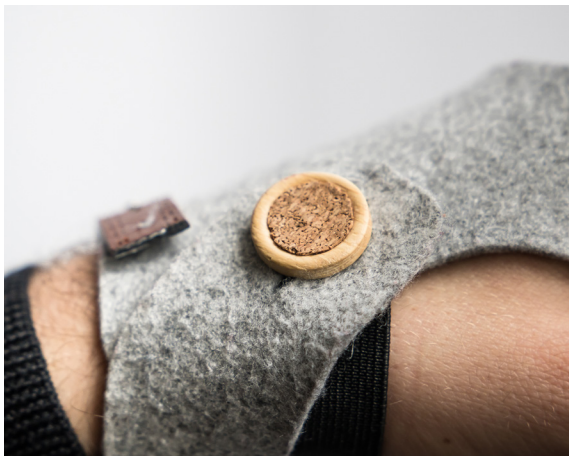
Fig 6.9 | When urging the user to exercise, the button will vibrate
